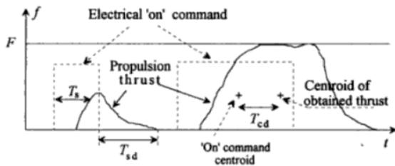
Figure 3. Thrust pulse in time domain (from [24])
