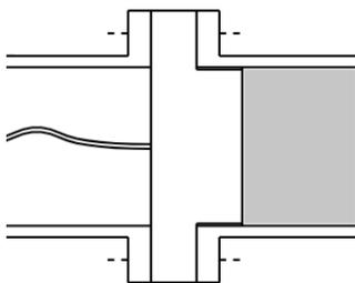
Figure 7. Injector/decomposition chamber interface
