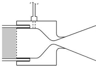
Figure 6. Decomposition chamber/nozzle interface
