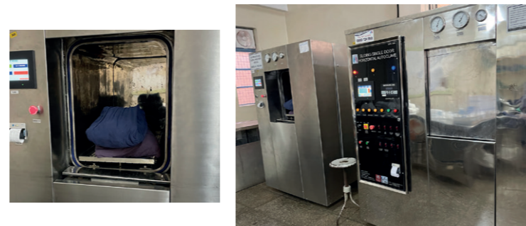
Fig. From left a) Packing within the autoclave b) running the autoclave
