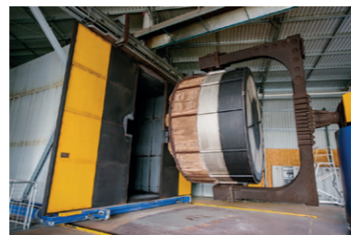
Fig. Rotational moulding of a large plastic product (Image credit: Global Rotomoulding)
