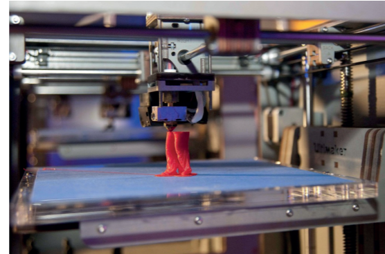
Fig. A complex form being 3D printed. (Image credit: Science museum)
