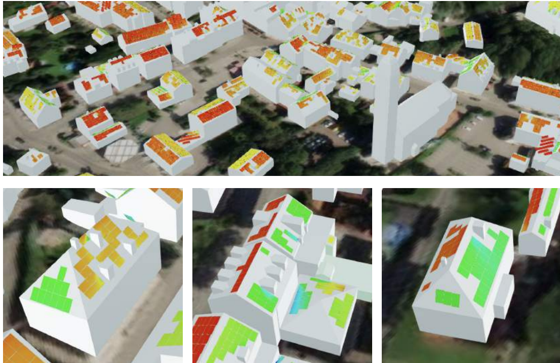
Figure 5.32: Example of buildings' PV potential assessment applied to Wartenberg model, visualization Cesium. Source: Willenborg 2022
