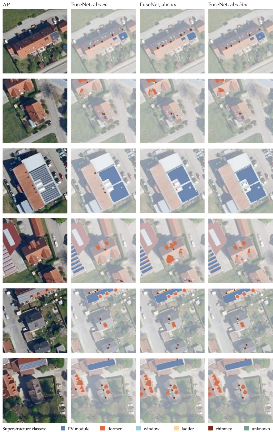
Figure E.5: No interpolation versus nn interpolation versus idw interpolation (FuseNet id-i, ii, and iii)
