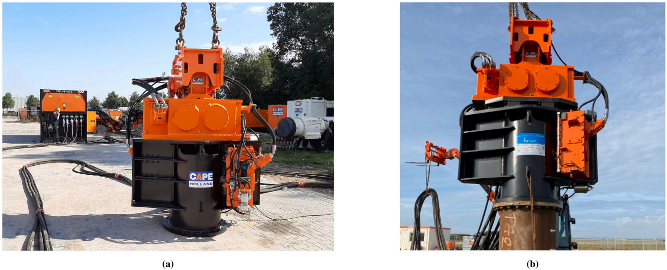
Fig. 1. The GDP shaker: (a) view at the manufacturing site; (b) shaker connected to a test pile via a bolted flange connection.
