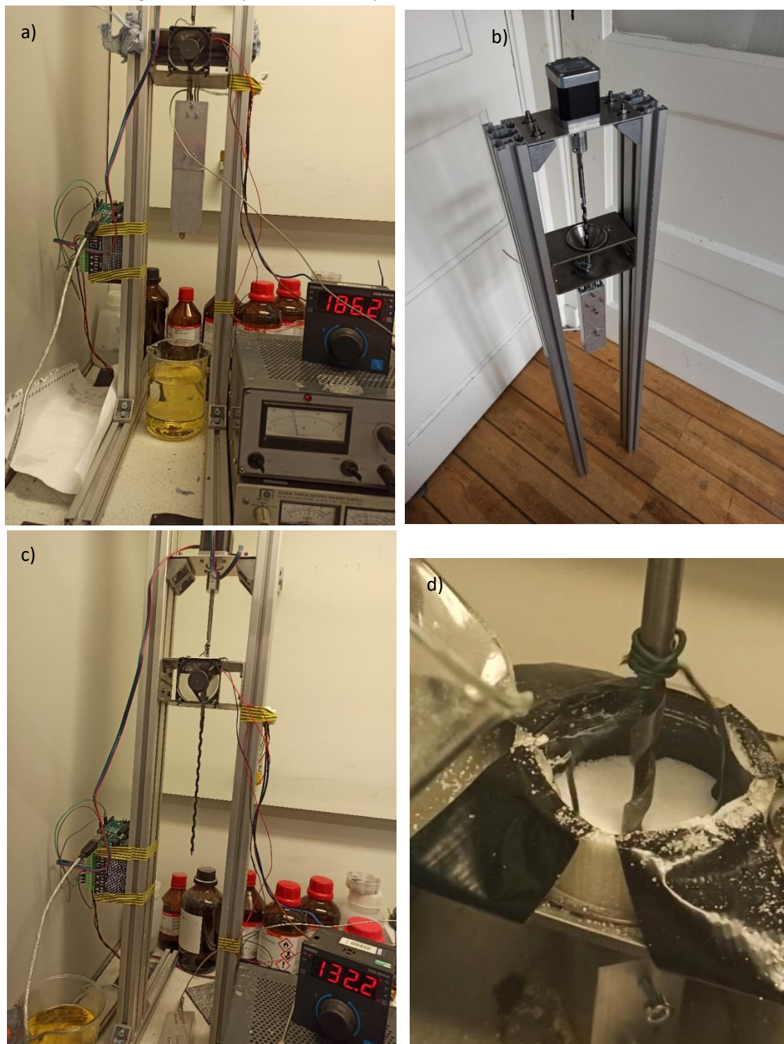
Figure 80: a) and b) show the experimental prilling setup. The suspension is mixed as a power, and filled in the funnel. The screw will transport the material down through a heater, which will melt the suspension. When it is melted, the screw will press the molten substance through a nozzle at the bottom, where it will form droplets. c) shows the screw which is inside the heating element and d) shows the improvised scraper.
