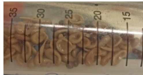
Figure 32: flat prills due to the impact with oil.
