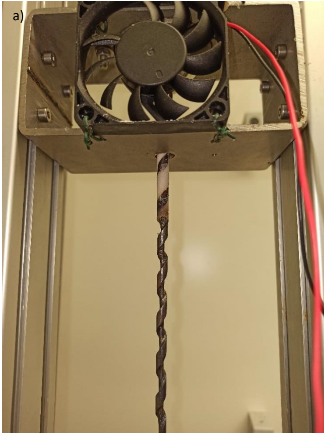
Figure 81: in a) and b), the part in the screw that is clogged is shown. Around this point, there is enough heat to partly melt the material, but since the screw is cold, it will attach to there. This will lead to a hard lump, where powder won't go through.
