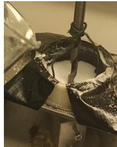
Figure 29: the added scraper (green wire), in order to improve throughput of the powder.
