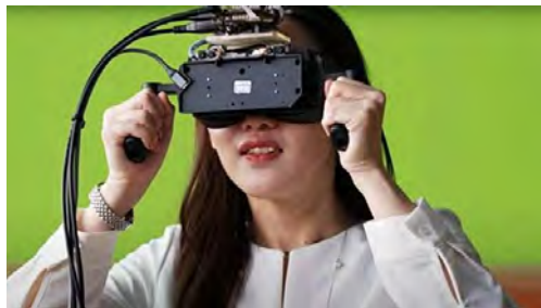
Figure 8: Wired prototype of an 8K VR headset by Sony, intended for business, medical and industrial applications (image source: Fahey, 2021).
