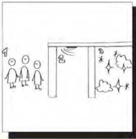
7 Visitors can enter 'bonus' exhibit space through a special entrance, consisting of the following sequence: A series of two sliding doors, a people counting sensor, an RFID gate reader. The 'airlock' style entrance will prevent visitors without access from entering the 'bonus' exhibit space.
