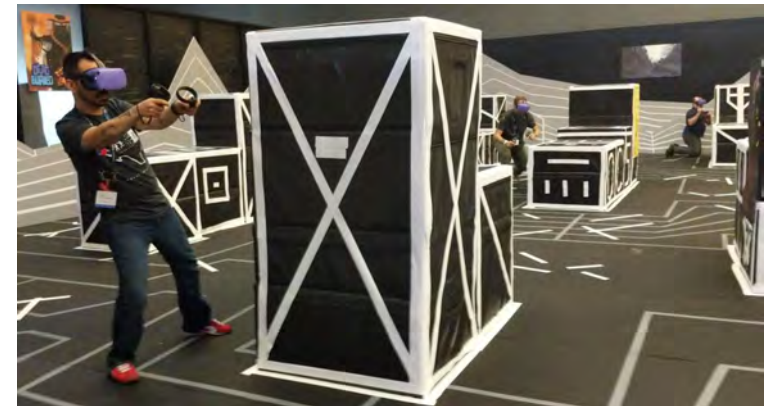
Figure 10: Wireless VR headset (Oculus Quest 2) being used for a mixed reality arena-scale multiplayer shooter game (image source: UploadVR, 2018).
