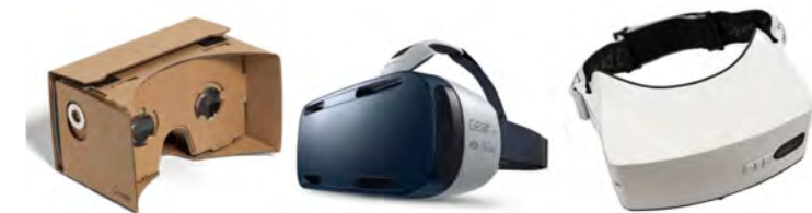
Figure 11: Three mobile-powered HMDs: the Google Cardboard, the Samsung GearVR Innovator Edition and the Gameface Mark IV (image source: Anthes et al., 2016).
