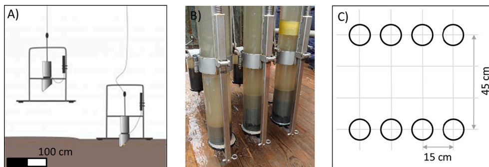
Fig. 5. (a) SPI deployment sketch (VLIZ 2022), (b) Photo of Multi Corer with collected sediment samples, (c) MC array with indication of dimensions.
