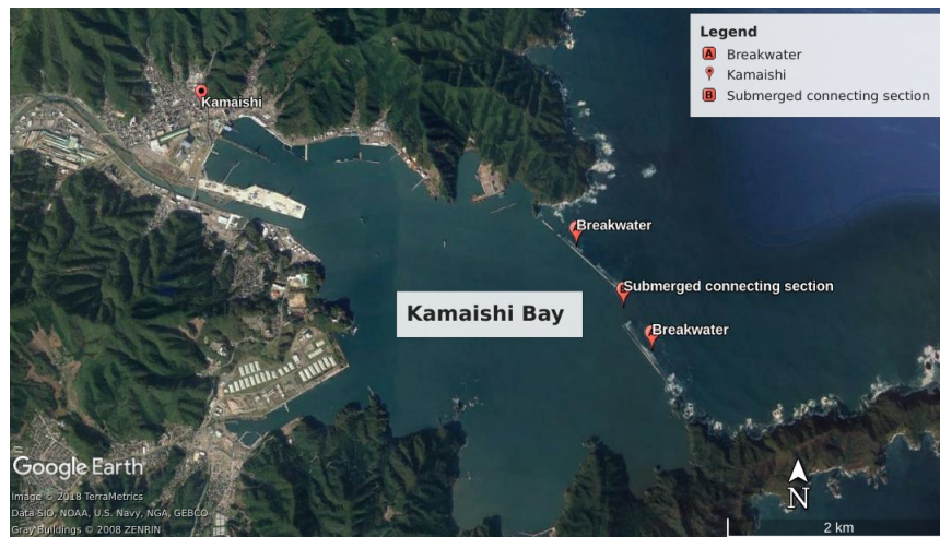
Figure 1: Kamaishi bay along with its breakwaters. The two breakwaters are separated by a submerged connecting section.
