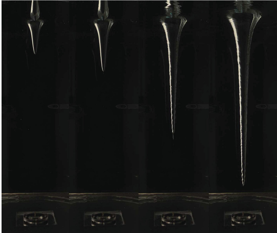
Figure 11 Free-surface vortex air core depths H_D for series 5 to 8 with from left to right: H_D = \pm 0.17 m, \pm 0.26 m, \pm 0.54 m and \pm 0.85 m. All air cores are typically funnel shaped
