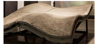
FIGURE 89 3D printed Panel by Loughborough University (Kucharek, 2015)
