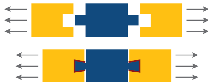
Figure 6.8: Examples of topological (top) and geometrical (bottom) interlocking when under tension (own work, 2024)
