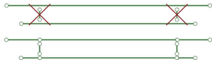
Figure 7.4: Segmenting horizontal lines to connect vertical lines (own work, 2024)
