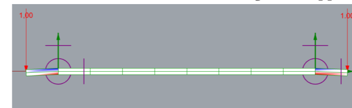
Figure 7.2: Deflection and stress on a beam with supports close to the load (adapted from Karamba3D, n.d.)
