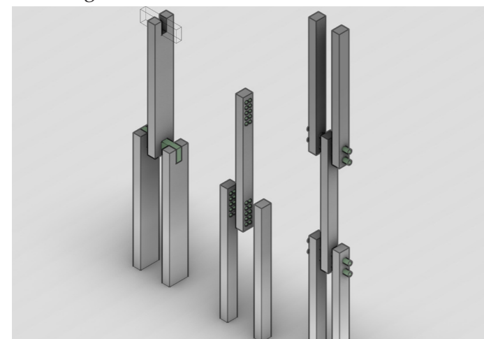
Figure 6.13: Vertical stacking of orthogonal beams with (from left to right) a) topological interlocking b) geometric interlocking c) dowels connection (Own work, 2024)
