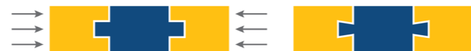
Figure 6.7: Conceptual examples of topological (left) and geometrical (right) interlocking (Estrin et al., 2021)
