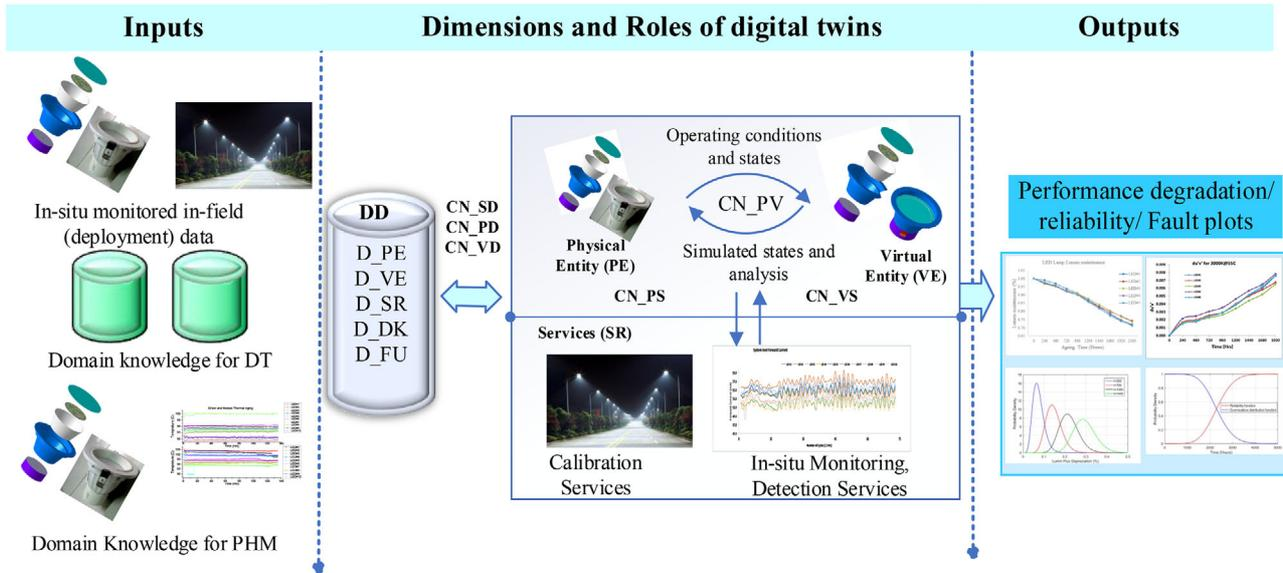
**Figure 25.** Digital twins implementation framework with the five dimensions (PE, VE, DD, CN, SR) for LED products. Adapted with permission.<sup>[229]</sup> Copyright 2018, Elsevier.
