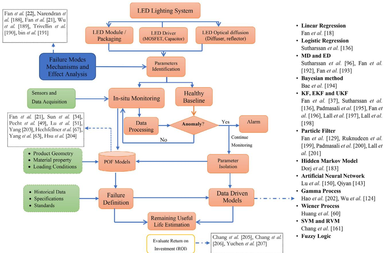
**Figure 23.** Fusion prognostics for LED lighting system. Adapted with permission.<sup>[20]</sup> Copyright 2014, IEEE.
