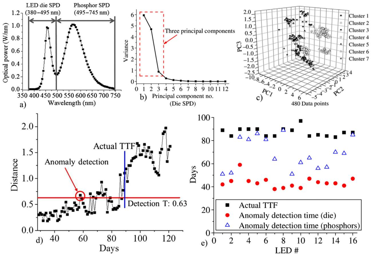
**Figure 16.** a) SPD feature extraction, b) principal components from extracted features, c) SPD training using KNN-kernel density-based clustering, d) distance measure from cluster centroid to detect anomaly, and e) anomaly detection using die SPD. Reproduced with permission.<sup>[157]</sup> Copyright 2014, IEEE.
