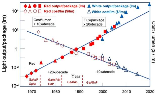
Figure 3. Haitz's Law demonstrating an increasing trend in luminous flux per package and decreasing trend in cost per lumen.<sup>[16]</sup>
