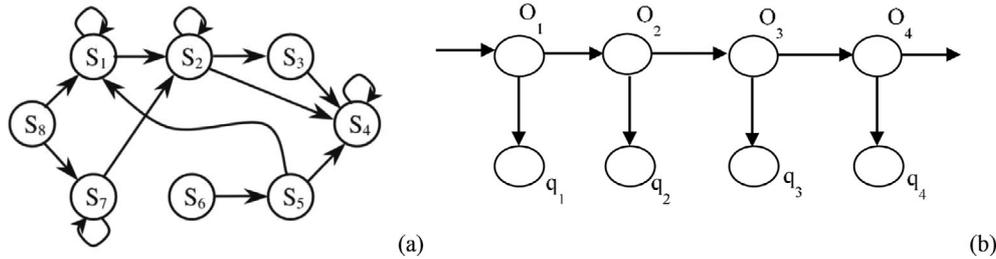
**Figure 22.** HMM graphical description: a) stochastic finite-state automation view of a HMM and b) a directed graphical model (DGM). Reproduced with permission.<sup>[179]</sup> Copyright 2007, Taylor & Francis.
