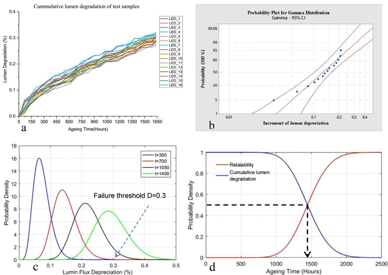
**Figure 11.** Gamma process: a) Average cumulative lumen degradation, b) probability distribution plots with gamma distribution, c) PDF at different times, and d) CDF and reliability plots. Reproduced with permission.<sup>[125]</sup> Copyright 2019, IEEE.
