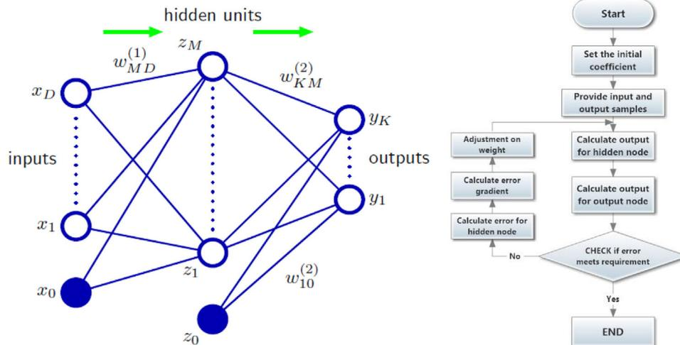
**Figure 13.** A representative network diagram for two-layer neural networks (left), flowchart for back propagation learning algorithm (right).
