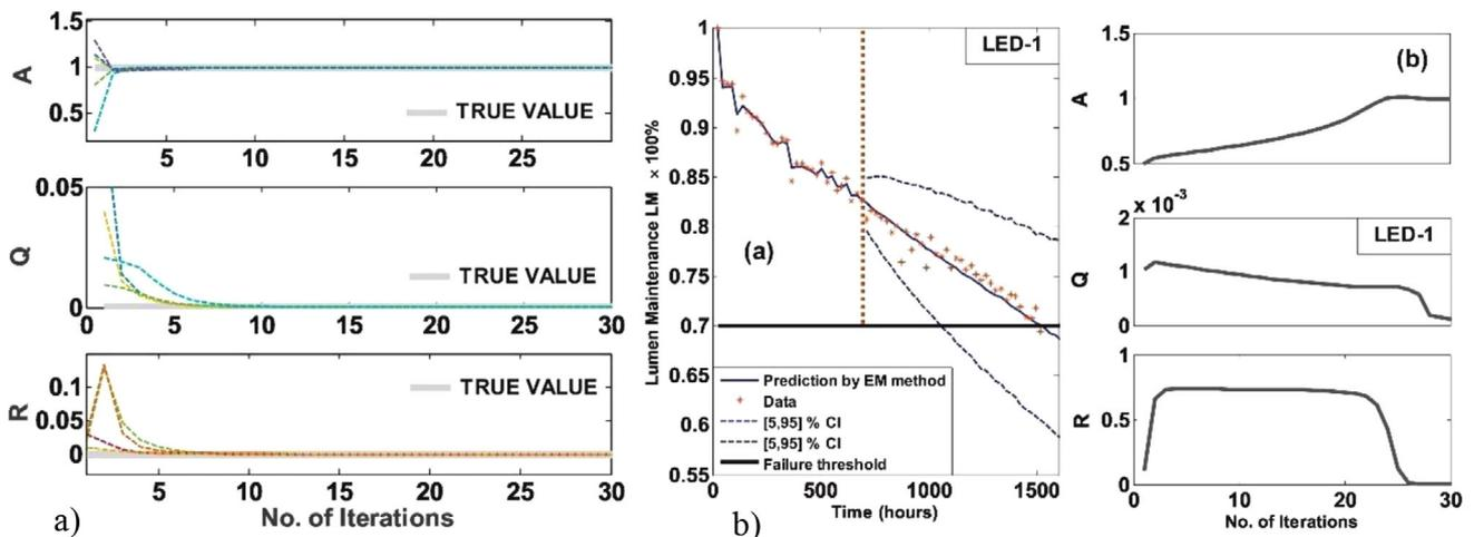
Figure 21. a) Parameter estimation using EM algorithm. b) RUL prediction based on EM estimated parameters and iterations trends values for parameters. Reproduced with permission.<sup>[177]</sup> Copyright 2018, Elsevier.
