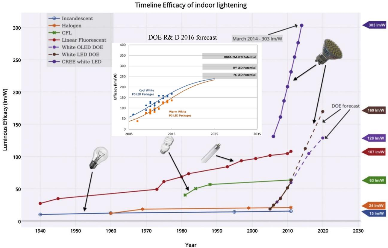
Figure 2. Development trends of lumen efficacy for different light technologies at normal working condition.<sup>[12,13]</sup>
