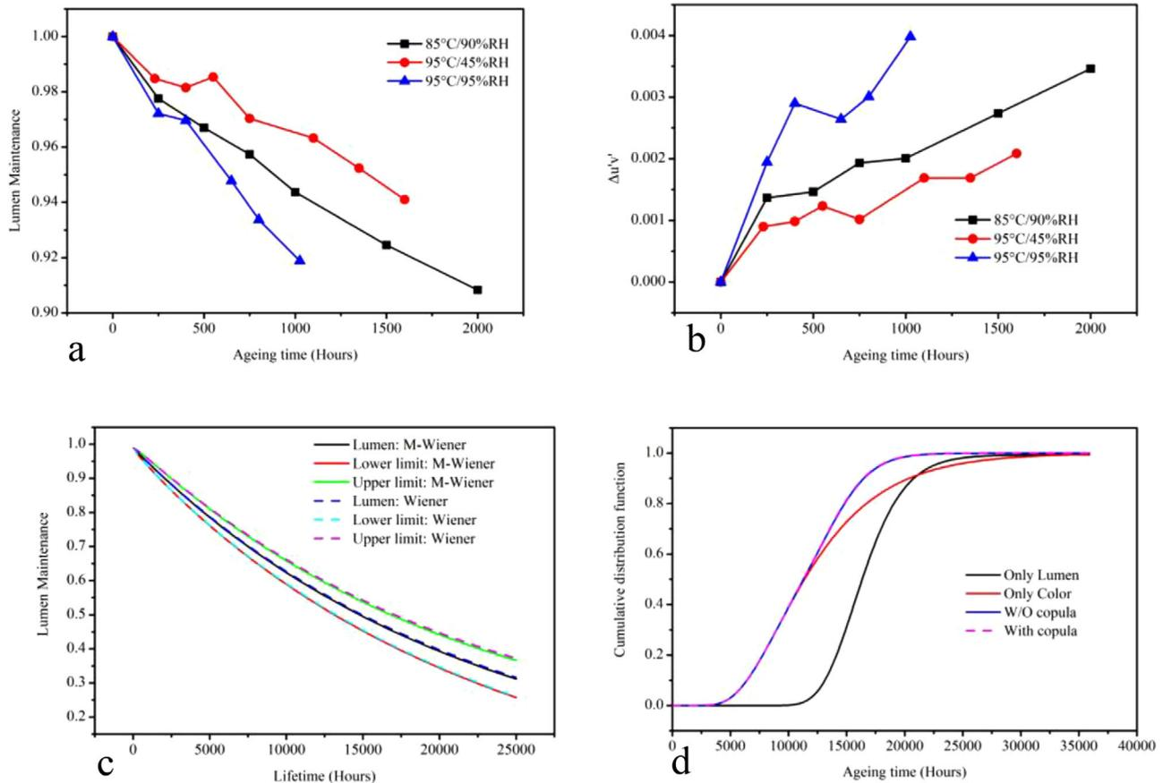
**Figure 10.** a) Luminous flux degradation, b) chromaticity shift, c) fitting lumen degradation data and lower and upper limits for Wiener process (WP) and modified WP, and d) cumulative distribution function for lumen and color with and without copula. Reproduced with permission.<sup>[60]</sup> Copyright 2015, The Optical Society.
