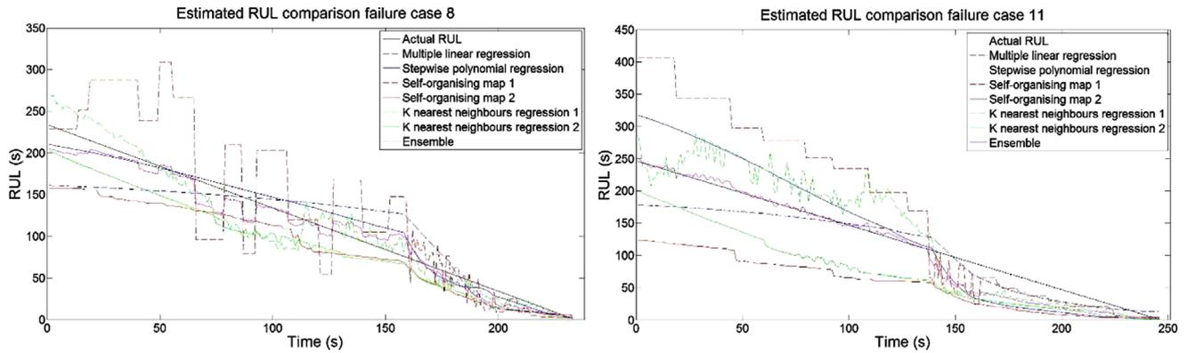
Figure 20. RUL estimation based on SOP, KNNR, multiple linear regression, and ensemble methods. Reproduced with permission.<sup>[156]</sup> Copyright 2018, Elsevier.
