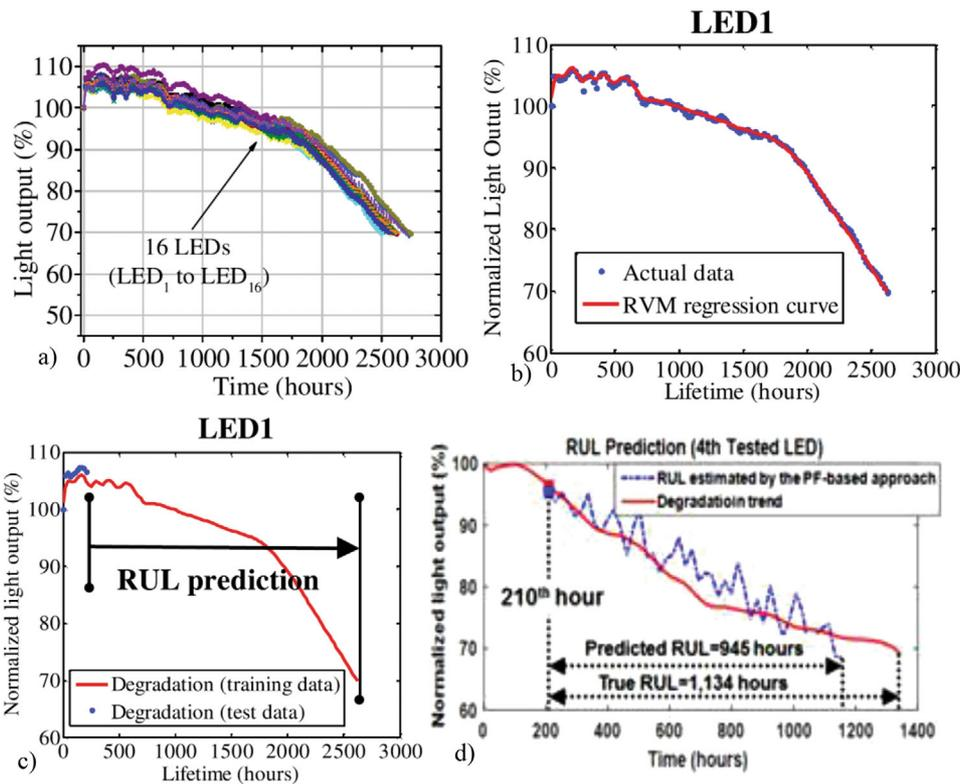
**Figure 17.** a) LED luminous flux degradation, b) parameter measurement for RUL, c) lumen degradation the RVM regression model, and d) PF-based lifetime prediction results. Reproduced with permission.<sup>[161]</sup> Copyright 2017, IEEE.
