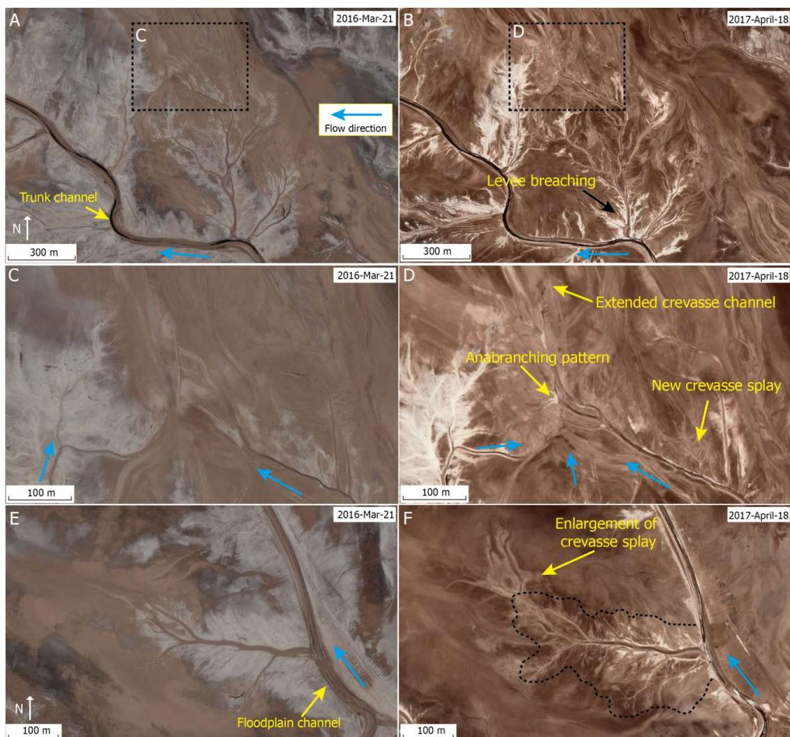
**Figure 7.** Examples of the enlargement of crevasse splays in the middle reach of the trunk channel (A,B) and floodplain channels (C–F) between 2016 and 2017 (for location, see Figure 1D). (A–F) are WorldView images from Google Earth. (B,D,F) indicate enlargement of crevasse channels and splays and levee breaching leading to formation of new splays during the 6 January 2017 extreme flood event. Blue arrows indicate flow directions.
