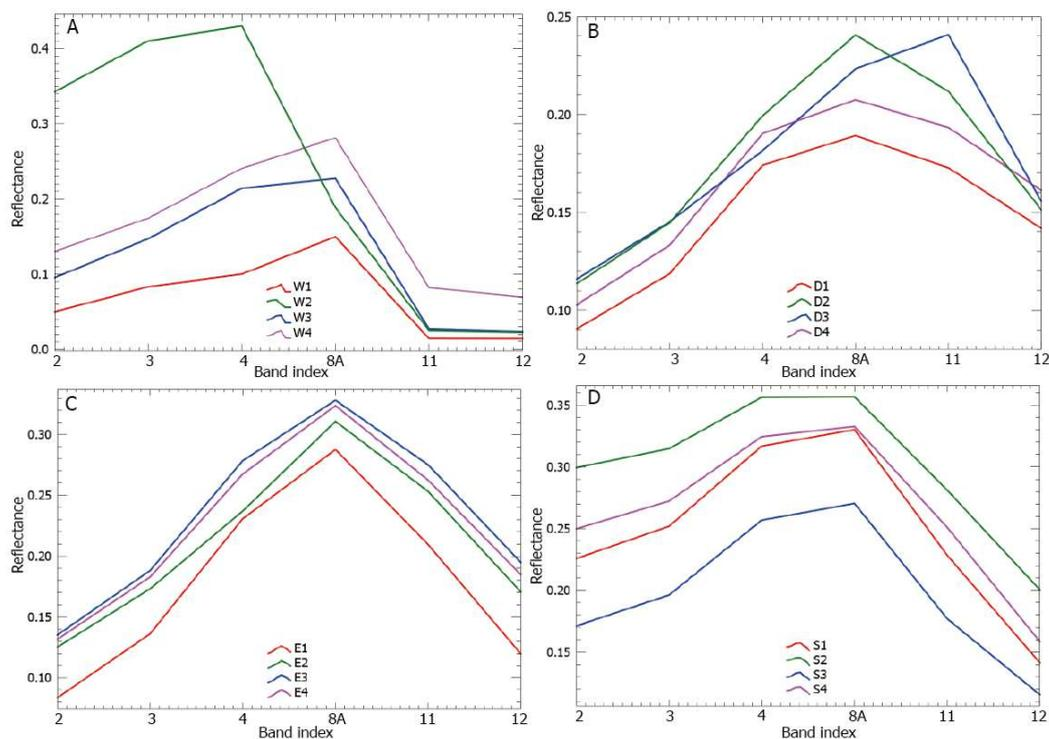
**Figure 5.** Spectral reflectance of different surface materials. (A): water; (B): dry land; (C): wet land; (D): salty surface. Letters in Figure 1D indicate the locations for the different lines shown on each graph.
