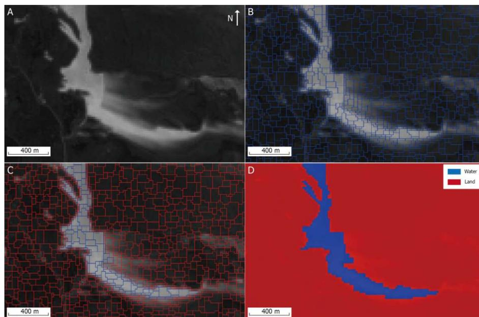
**Figure 4.** General steps of the multiresolution segmentation procedure used to extract water bodies from MNDWI results. (A): part of MNDWI results in the study area; (B): results of the multiresolution segmentation on MNDWI results; (C): results of classification based on Otsu's threshold value. Red polygons indicate land while blue polygons show water; (D): view of classification results.
