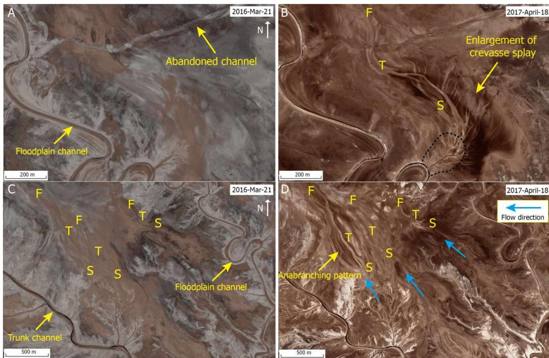
**Figure 10.** Examples showing the development of erosion cells. Letters S, T and F represent the scour, transport and fill sections in the erosion cells. (A,B) show the interplay between the enlargement of crevasse splays and erosion cell development in association with an abandoned channel. (C,D) indicate erosion cell development in a topographic low between channels, illustrating how anabranching networks of channelized sections may form during the flood peak.
