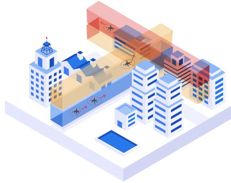
Figure 3.3: Isometric view of layers at intersections, configured such that cruising aircraft do not interfere with each other, and turn layers always at the same altitude.
