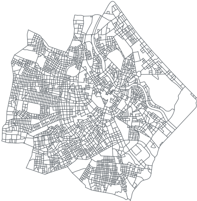
Figure 5.6: Constrained airspace structure extracted from the street network of the city centre of Vienna.
