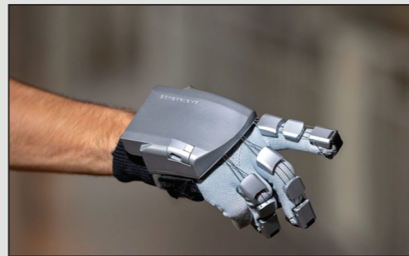
Fig 11 SenseGlove implements an array of pressure sensing techniques to enable physical feedback for XR (SenseGlove, 2023).
