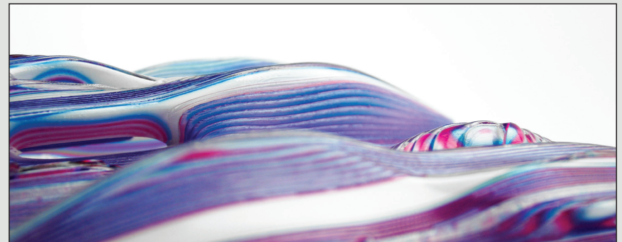
Fig 5 Multi-Material Jetting can create complex three-dimensional material structures (Illusory Material, 2020).
