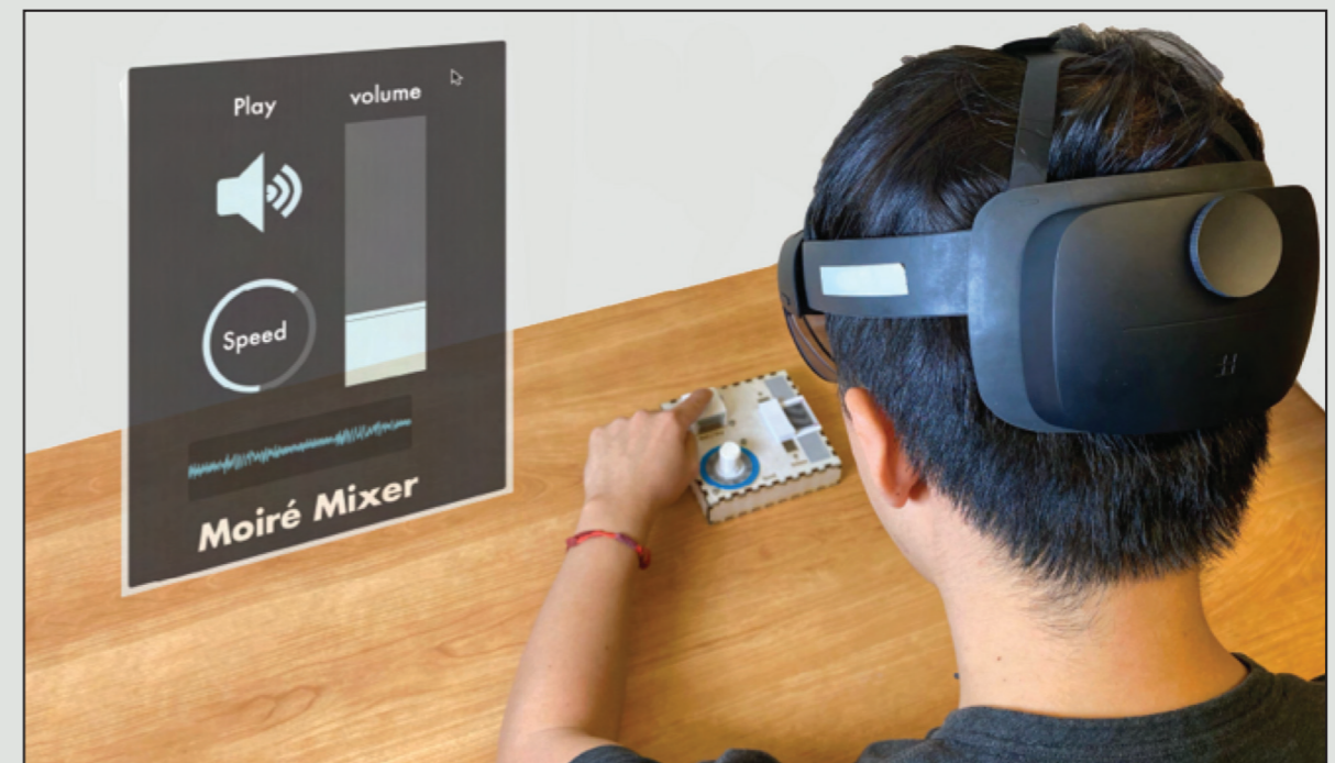
Fig 20 Virtual sound interface controlled through Physical MoiréWidgets (Zamora et al., 2024).
