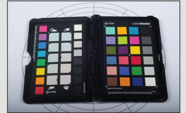
Fig 93 X-rite color checker passport and calibrite software were used for color calibration.
