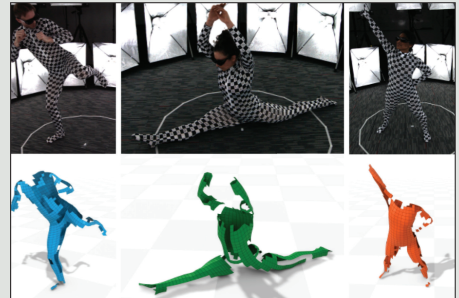
Fig 43 Markers on contouring edges are not recognized as a result of viewpoint distortion (Chen et al., 2021).
