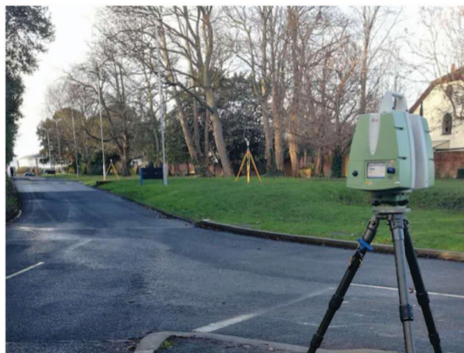
Fig. 9. (Color) Leica P20 Scan Station at the data collection site.
