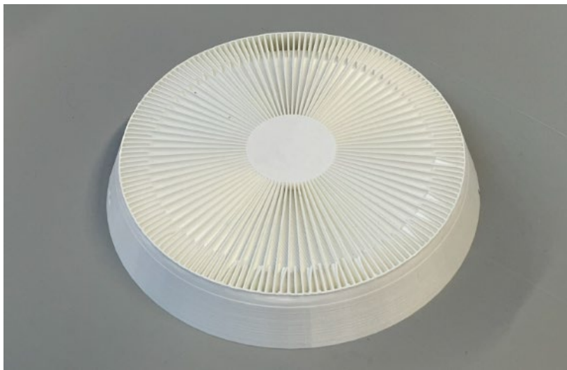
Figure 53 - 3D printed PLA model that was made prior to prototype 1 production.
