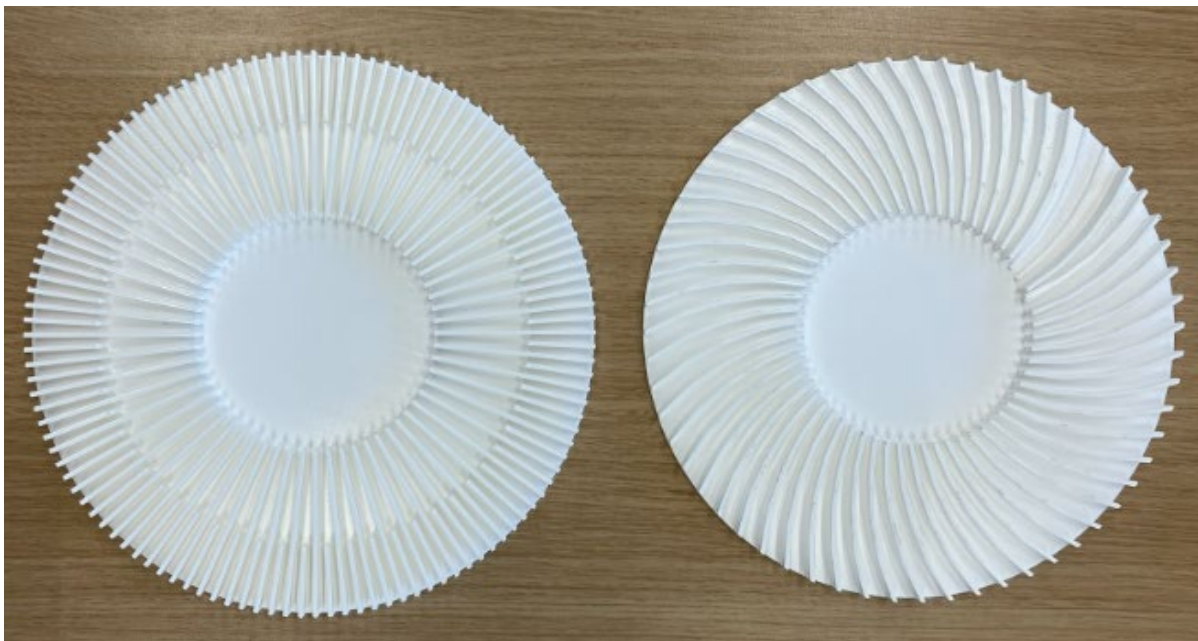
Figure 28 - left: peripheral fins, right: winding fins.
