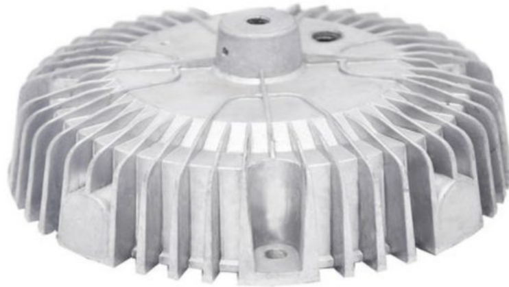
Figure 7 - example casting of the 390 alloy. This alloy is used for engine blocks, valve bodies and piston housings which require a certain level of thermal durability.
