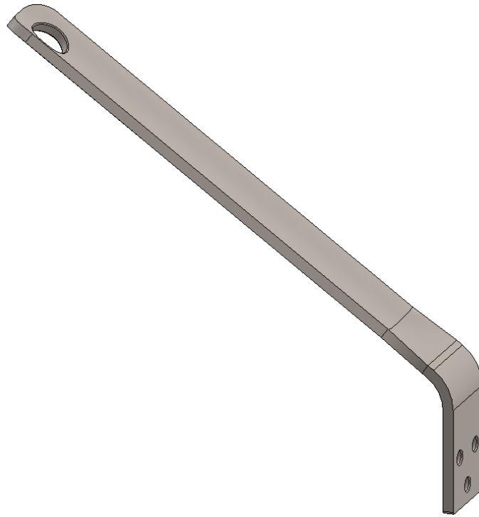
Figure 14 - metal strip after bending operation.
