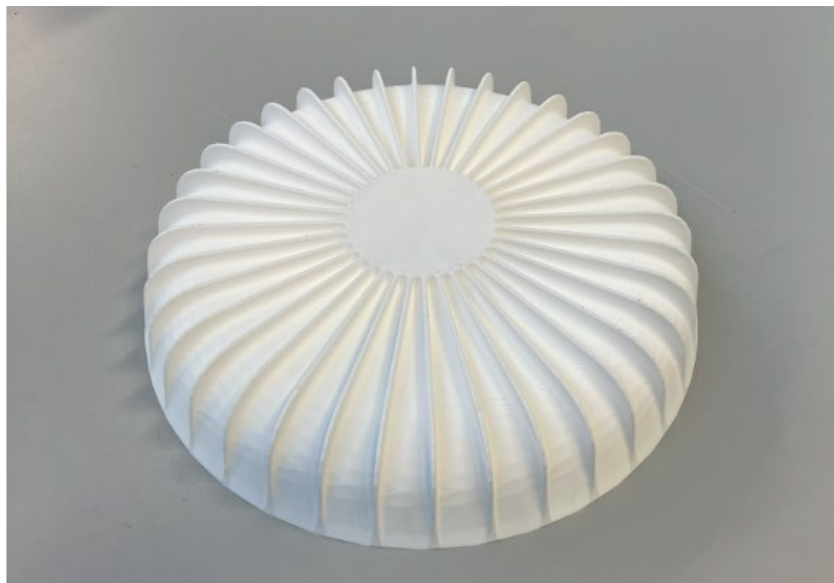
Figure 54 - 3D printed PLA model that was made prior to prototype 2 production.
