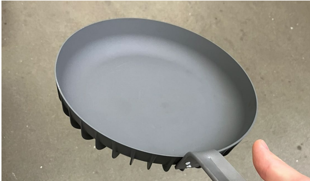
Figure 8 - the second prototype (V2) right after anodizing.
