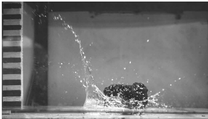
(a) Video still of a polymetallic nodule colliding with the wet steel plate. The nodule is about to break into a few large pieces, and there will be a limited amount of debris.
