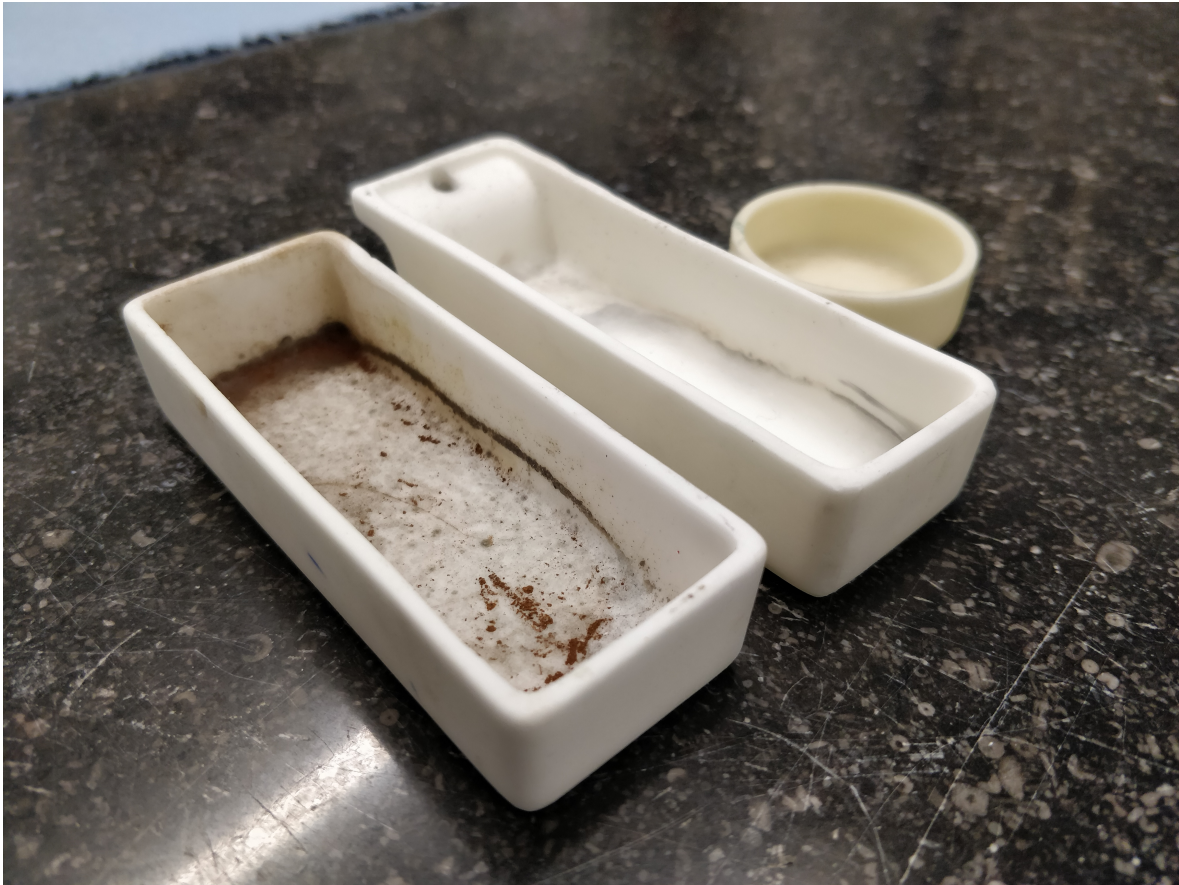
Figure 6-2: Overview of the alumina crucibles used. The crucibles will be referred to as a boat crucible, a hooked crucible, and a round crucible. Sizes are 8x3x2, 9x3x2, and 3.5x1-1.25.
