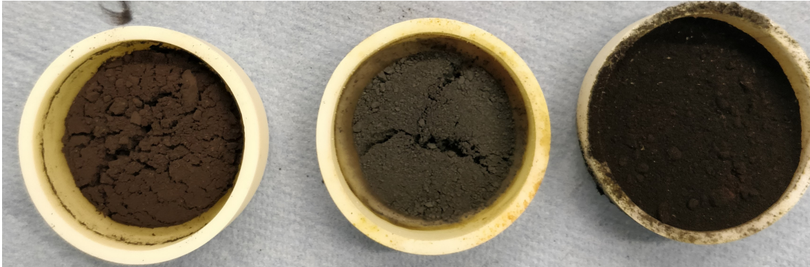
Figure 7-5: Goethite, BOF dust, and BF dust. During treatment, the dust undergo sintering.
