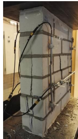
Figure 4: Compression tests on the companion masonry wallets: (a) stress-strain curve; (b) typical observed crack pattern.
