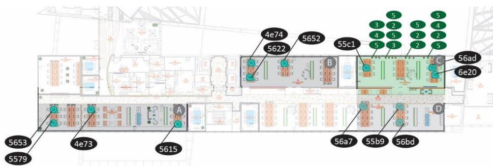
Figure 50. Pilot floor E03 measurement devices.
