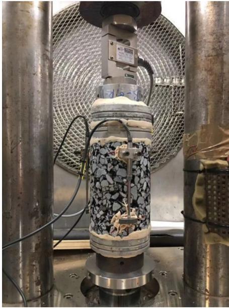
Fig. 9. Uniaxial cyclic compressive tests for PA mixes.
