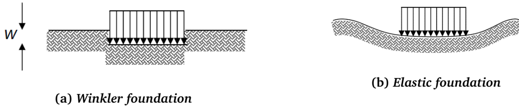
Figure 1.2: Differentiating the soil behavior in Winkler and Elastic foundation models [33]
