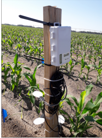
Figure 2.4.: 3 leaf wetness sensors installed at a wooden pole at early stage.
