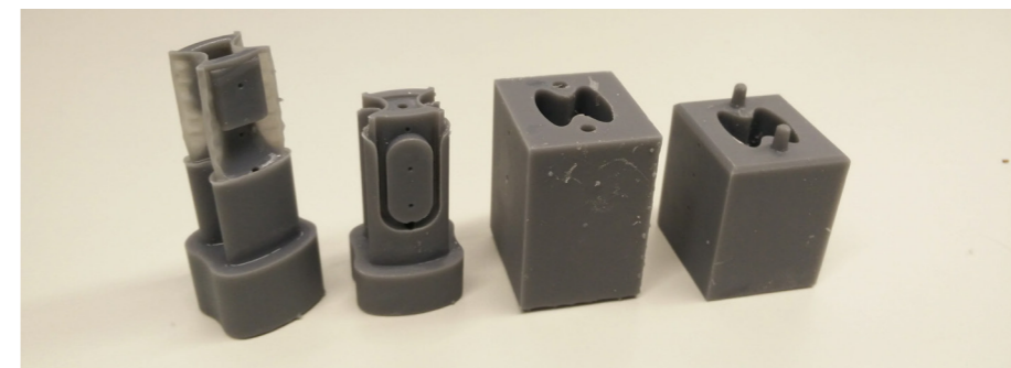
Figure 34: Moulds created for prototyping soft part of probe and to check feasibility of manufacturing
