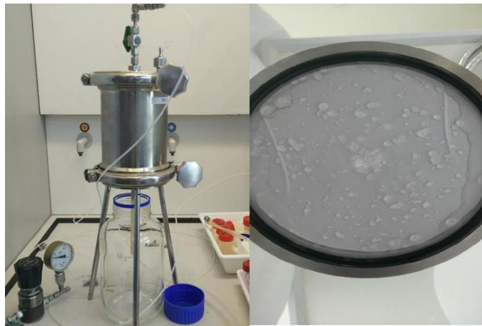
Figure 2.7- Filter setup to filter polymer (left), filter(right).
