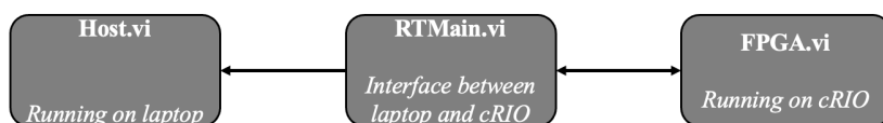
Figure C.1: Schematic showing the interface between FPGA, RTMain, and Host VIs in LabVIEW.
