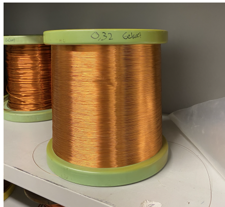
Figure B.4: Spool of enamelled copper wire with diameter equal to 0.32 mm used to connect the piezoelectric transducers in the experimental setup.
