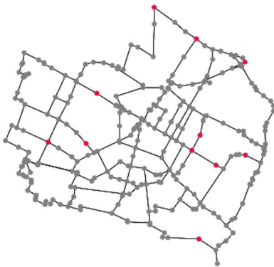
Five Reservoirs, Monitoring Network of Flow Sensors
