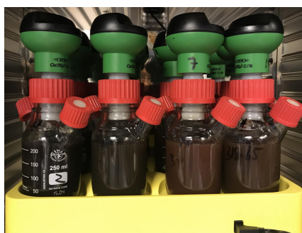
Fig 3.1 Oxitop devices used for measuring specific anammox activity and specific denitrification activity..
