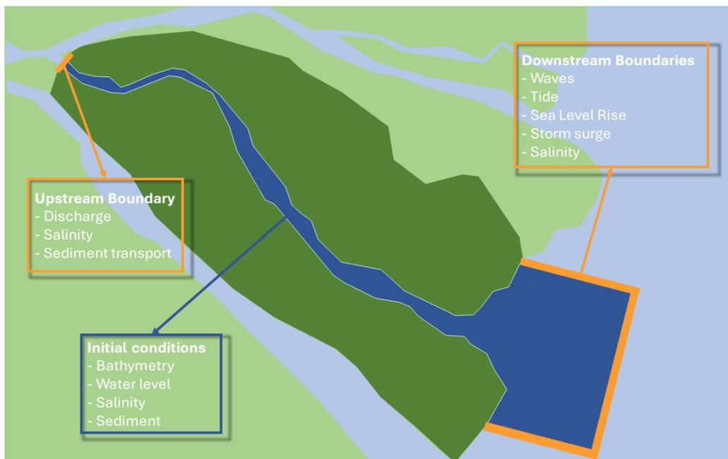
**Figure 5.1:** Conceptual Model; dark blue area indicates the part of the estuary in which the hydro- and morphodynamics are modelled, dark green area indicates the land that is part of the system of interest, orange contours mark the input boundaries of the hydraulic model.
