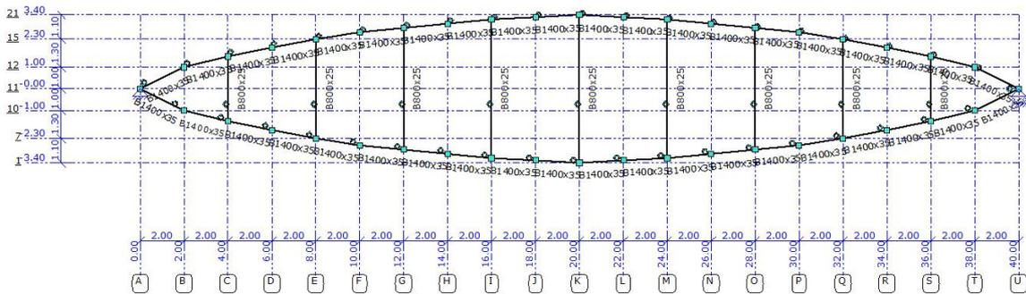
**Figure 7.9:** Top view of steel frame structure of the gate, showing the two arcs and nine horizontal girders.
