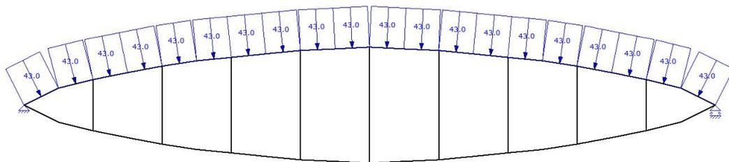
Figure E.12: Hydrodynamic load on the gate
