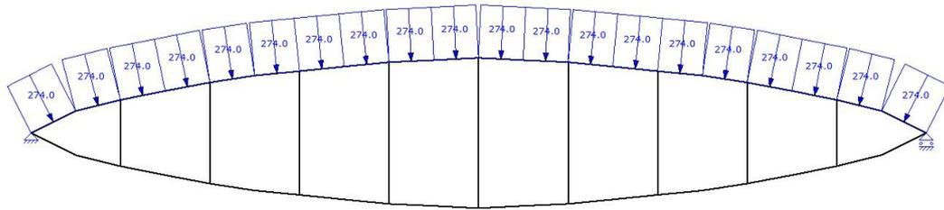
Figure E.11: Hydrostatic load on the gate
