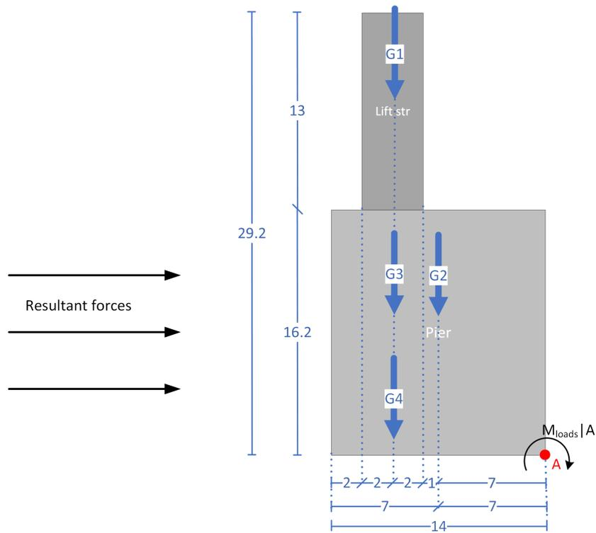
**Figure E.17:** Cross section with loads of the storm surge barrier for LC1
