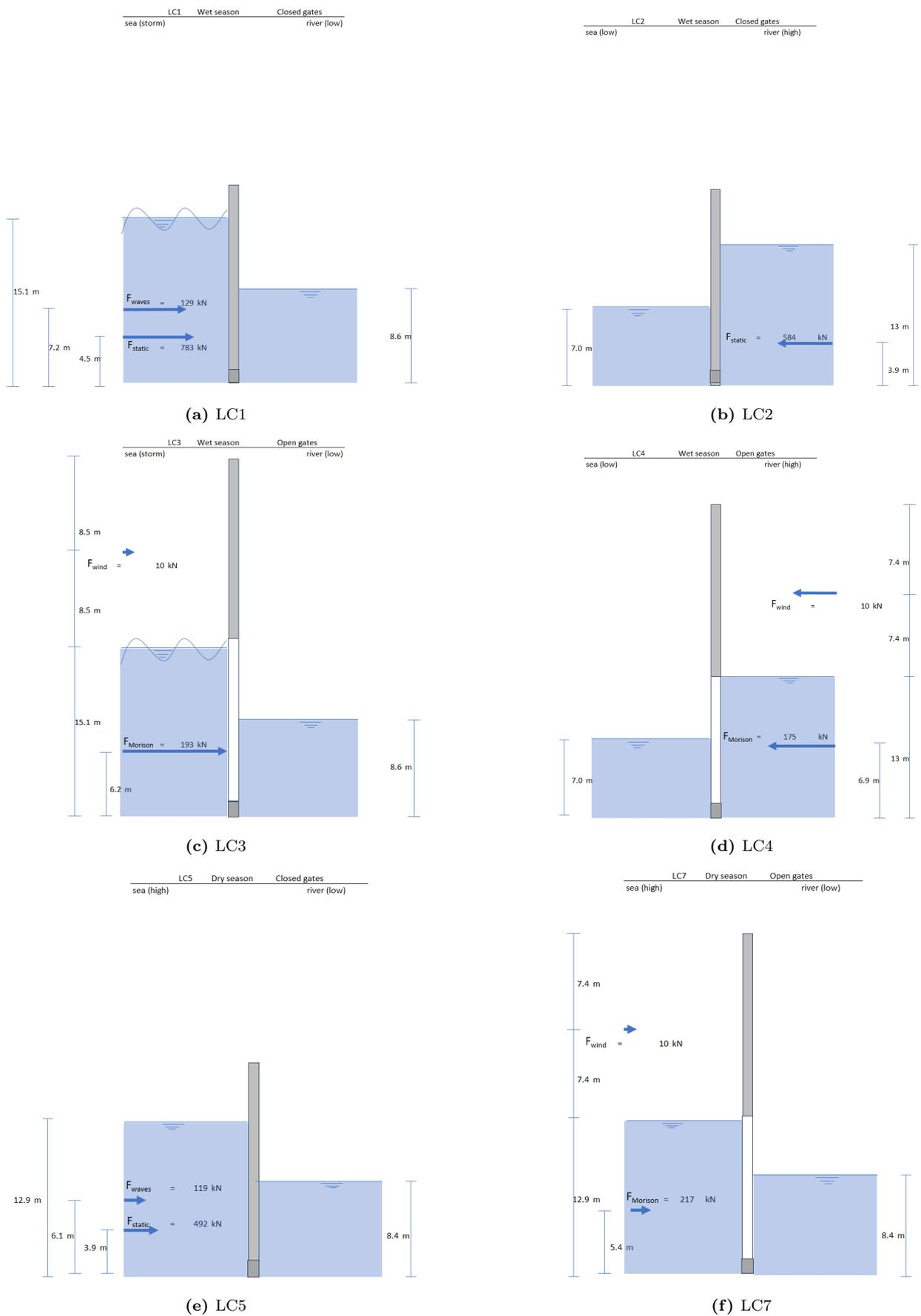
Figure 7.7: Complete load schemes for all critical LCs
