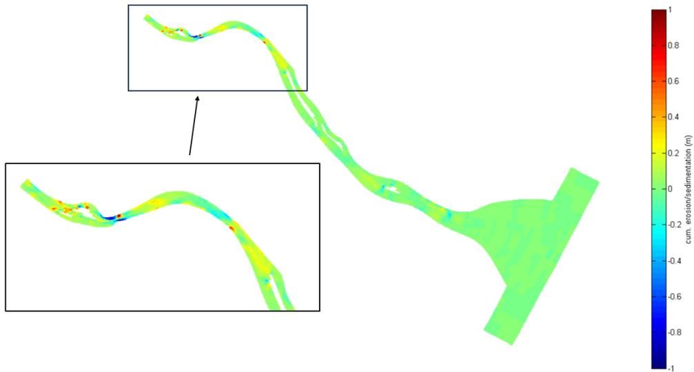
**Figure 6.6:** Difference in cumulative sedimentation/erosion between base year 2025 and 2100 without a barrier.
