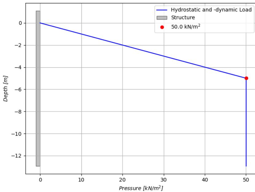
Figure E.9: Hydrostatic and -dynamic Load LC2
