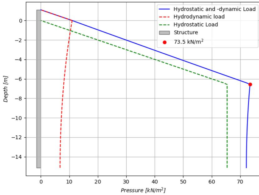
Figure E.8: Hydrostatic and -dynamic Load LC1
