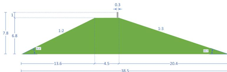
**Figure 7.1:** Cross-section of the sea dyke design, including dimensions of the height and width in m.
