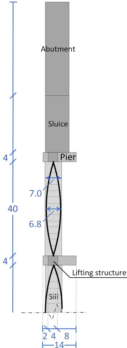
**Figure E.20:** Top view of the storm surge barrier with a potential sluice and abutment for future plans with unknown dimensions
