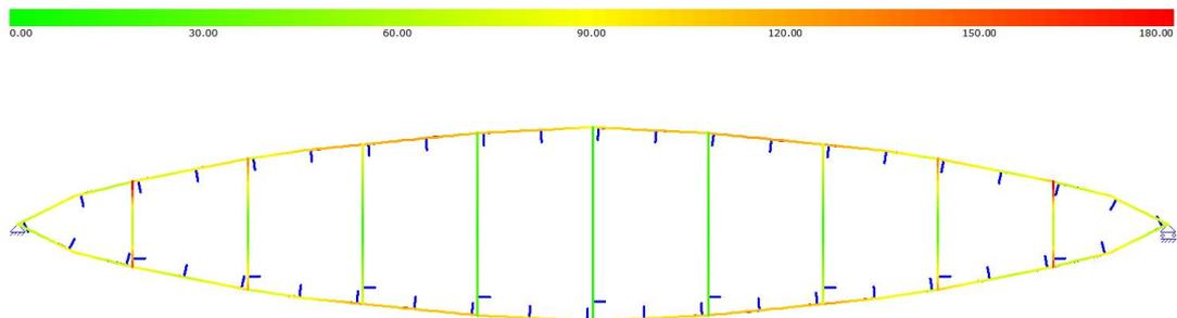
Figure E.13: Steel frame stresses
