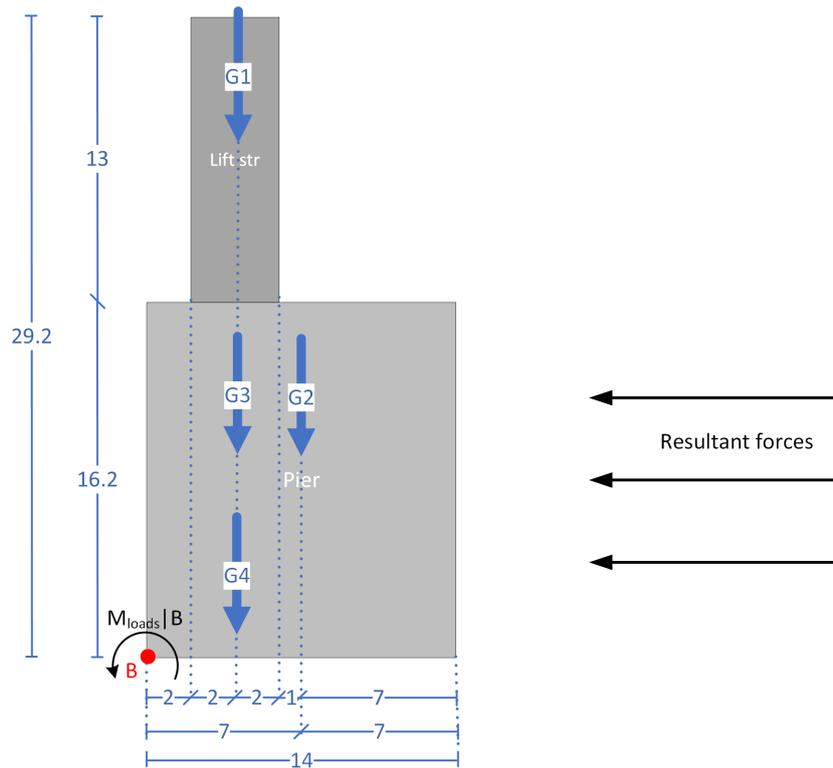
**Figure E.18:** Cross section with loads of the storm surge barrier for LC2
