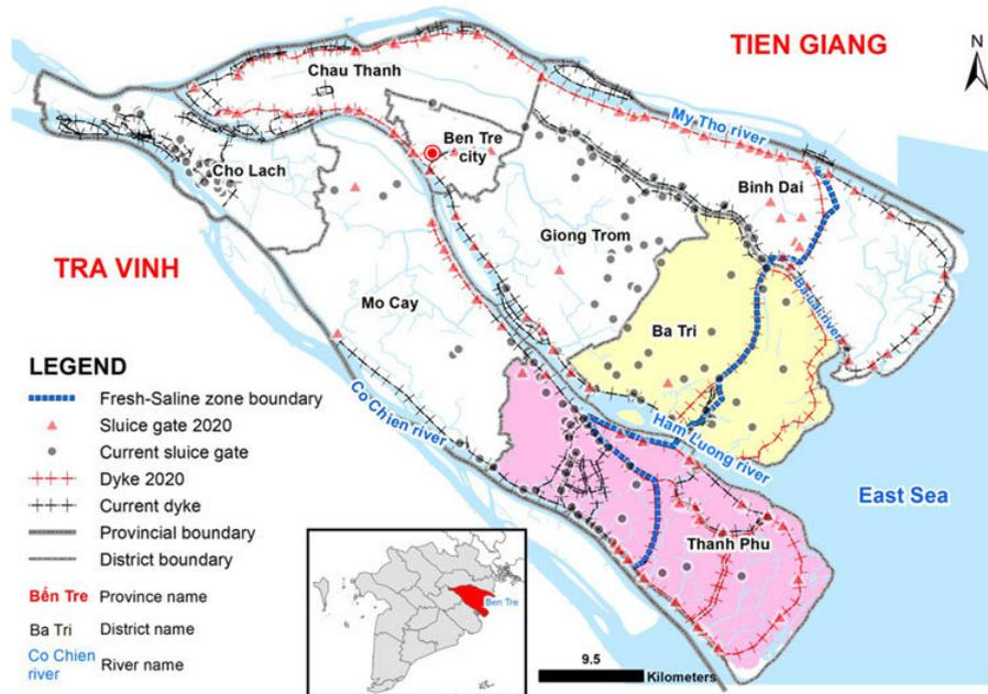
Figure 3.3: Ben Tre dyke protection and sluices (Korbee et al., 2019)
