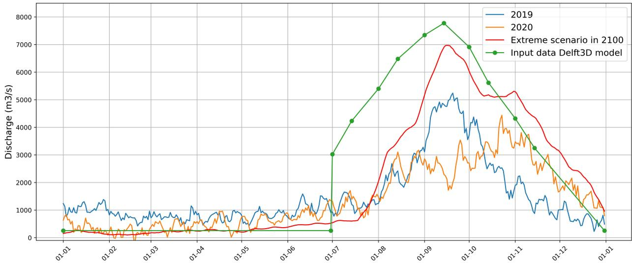
**Figure B.3:** Discharge time series in the Ham Luong estuary. Blue: discharge in 2019 based on My Thuan discharge. Orange: discharge in 2020 based on My Thuan discharge. Red: Extreme scenario in 2100 based on 2019 and 2020 data. Green: Input discharge data for the model.
