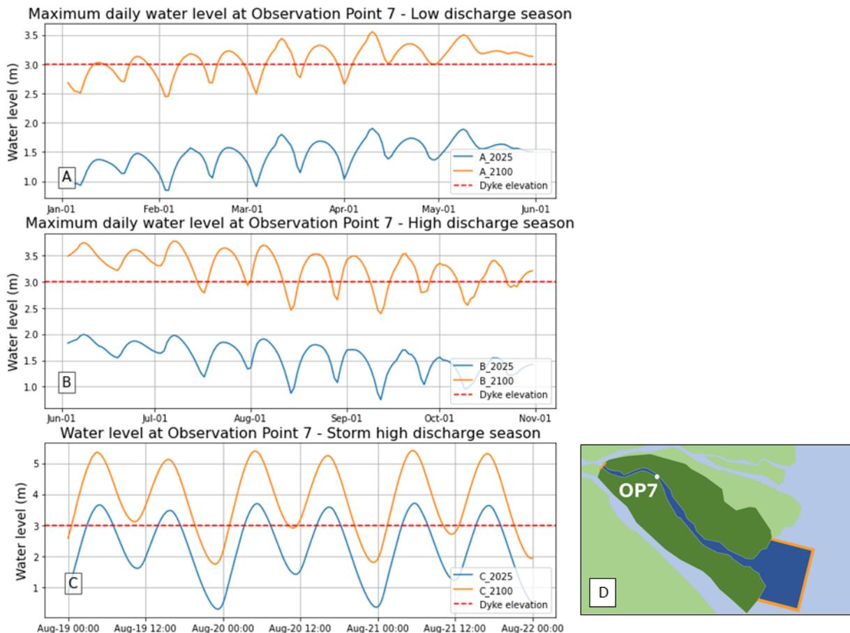
**Figure 6.1:** Water levels at observation point 7. A: The daily maximum water level at the observation point in the dry season. B: The daily maximum water level at the observation point in the wet season. C: The water levels during a storm at the observation point. D: Location of Observation Point 7.
