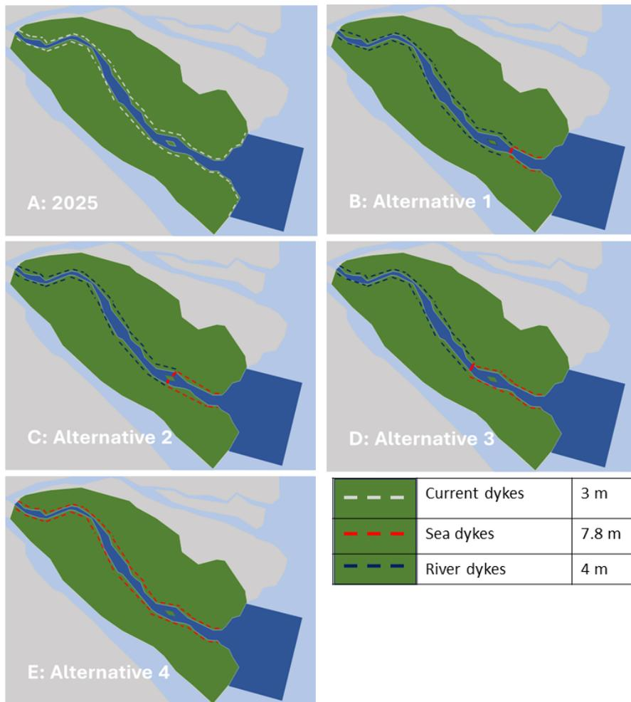
**Figure 7.2:** Dyke system: The existing dyke system for the current situation (A) and the proposed dyke systems for the four alternatives (B to E). The height of the sea dykes includes the 1.0 m height of the wall on top of the dyke
