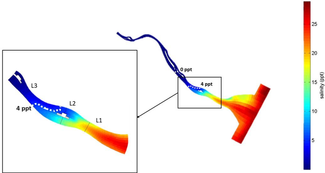
**Figure 6.4:** Maximum salt intrusion in 2100 during low discharge season in the Ham Luong River, with the 4ppt and 0 ppt boundaries in white
