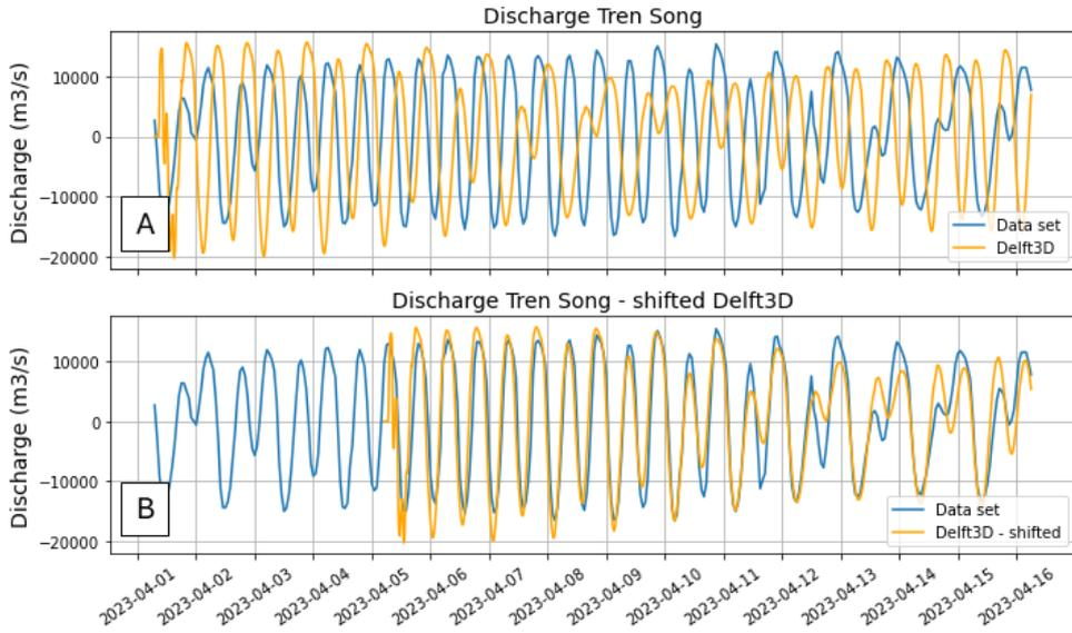
**Figure 5.4:** Comparison discharge from dataset to output of Delft3D. A: Discharge in Tren Song, dataset provided by SIWRP. B: Discharge in Tren Song, same datasets as in figure A except the Delft3D data is shifted 3 days 22 hours forward.
