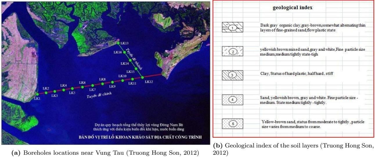
Figure E.6: Location and soil layers of boreholes
