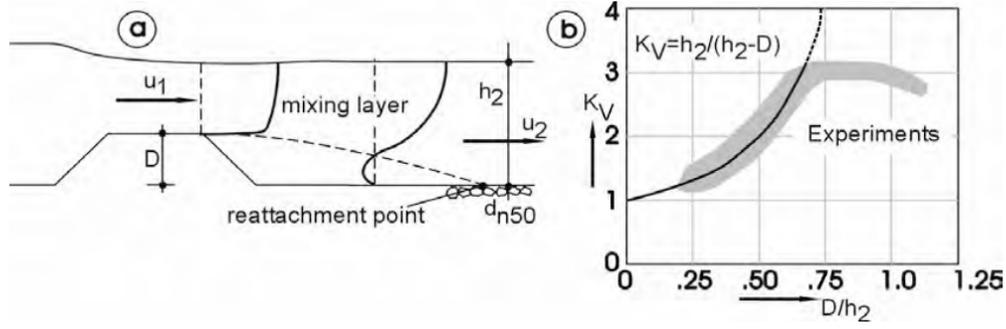
**Figure E.22:**  $K_v$  coefficient behind sill (Schierreck & Verhagen, 2012)
