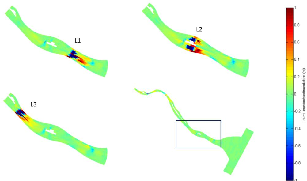
**Figure 6.7:** Differences in cumulative sedimentation/erosion between base year 2025 and three situations with barriers in 2100.
