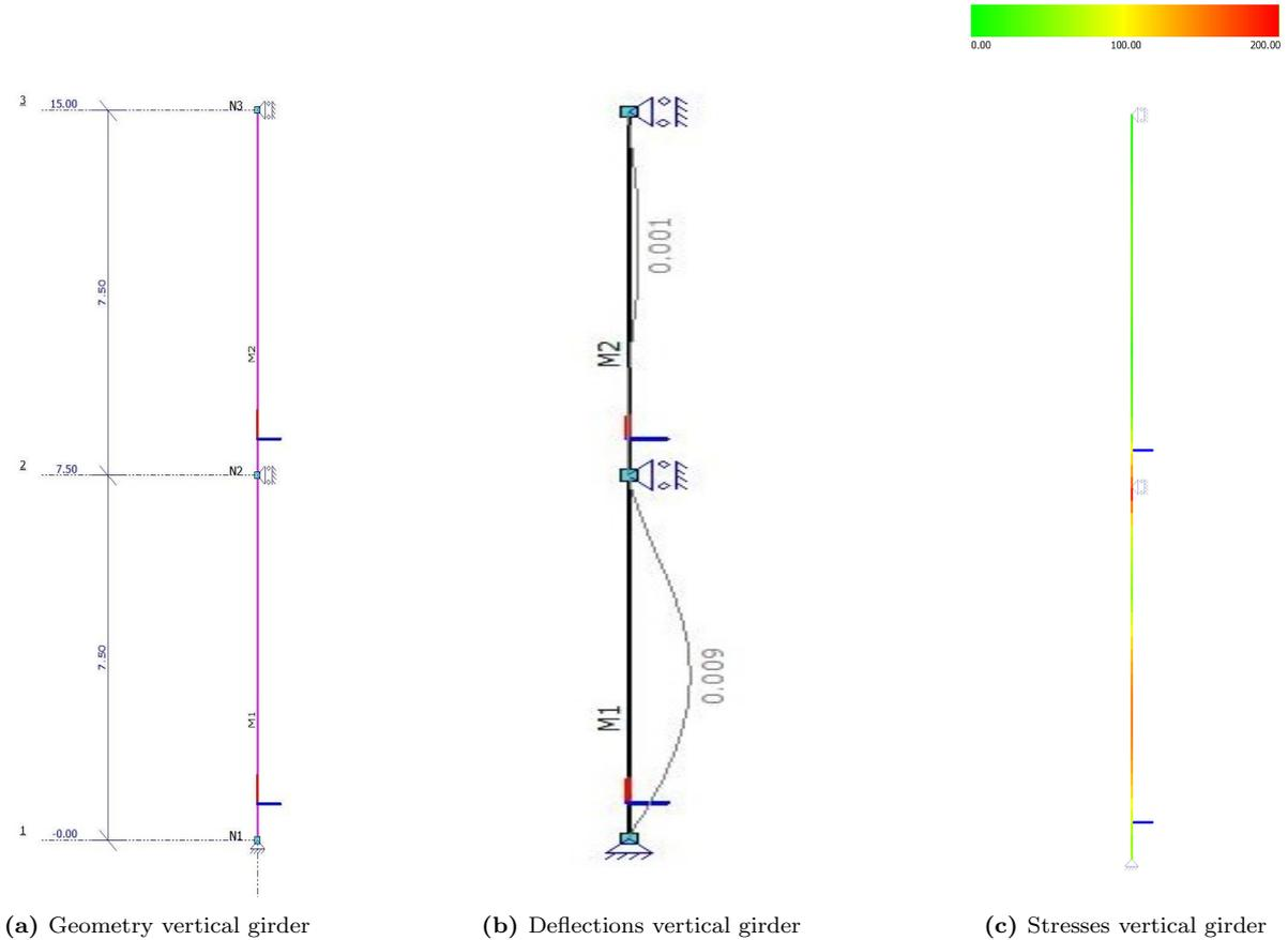
**Figure 7.10:** Vertical girder geometry, deflection and stresses
