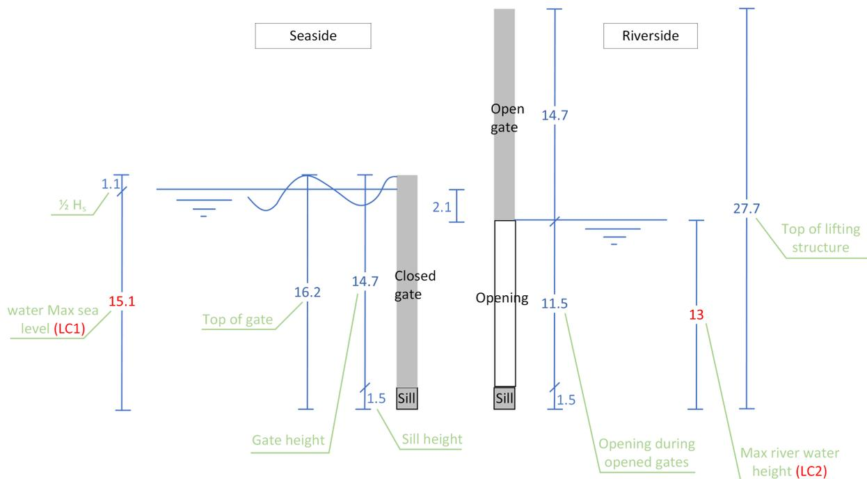
**Figure E.19:** The heights of the water and barrier during operation and rest. For this figure, the sea water level for LC1 is drawn on the left and the river water level for LC2 is drawn on the right, both in red. This is not an existing LC, but is used to explain complications during operation.
