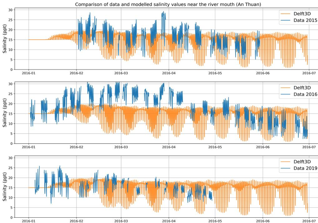
**Figure 5.5:** Verification salinity. Comparison between measured salinity values of three years and modelled salinity values.
