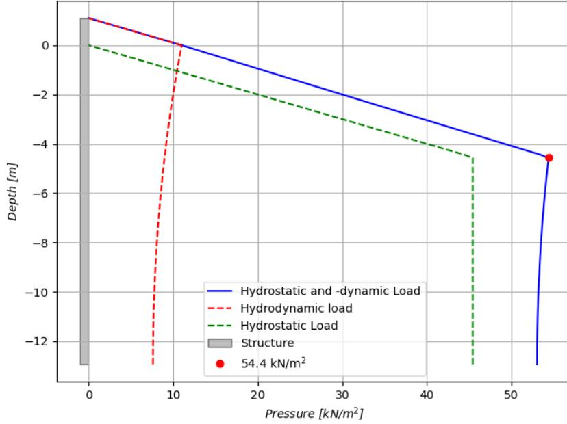
Figure E.10: Hydrostatic and -dynamic Load LC5
