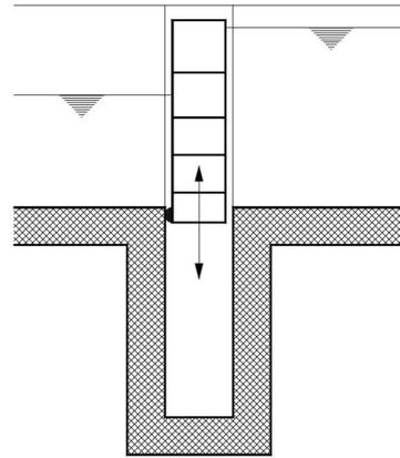
(b) Principal of a drop gate Source: (Kuijper et al., 1998)
