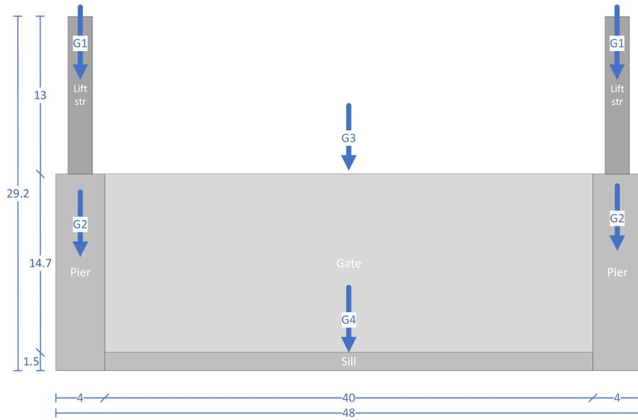
**Figure E.16:** Front view of the storm surge barrier
