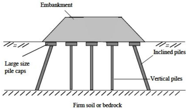
Figure 7.11: Piled embankment with batter piles, indicated as 'inclined piles' (Sakleshpur & Madhav, 2013).
