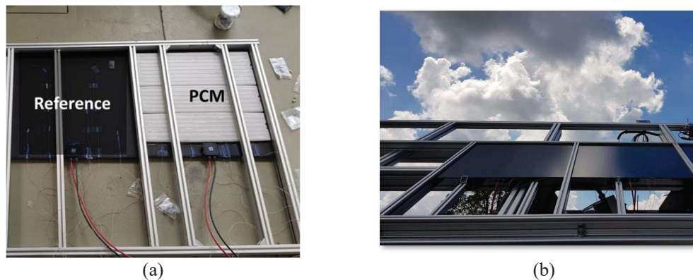
Figure 7(a) photographs the backside of the manufactured PV mini-modules for testing with the PCM slabs that are mechanically attached to one of them. (b) The IBC mini-modules, when installed on a tilted plane at an angle equal to 35°, have an appealing aesthetic aspect, with a homogeneous color and the cells barely visible.
