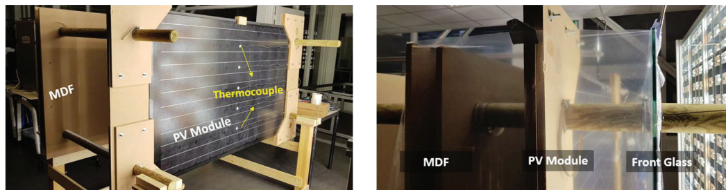
Figure 2 Simplified demonstrator of the PV chimney concept. Each layer measured 2.2 m in width and 1.02 m in height; measures fitting the size of the c-Si PV module utilized. The Concept was studied under controlled conditions inside the PV laboratory of the PVMD group at TU Delft, using a AAA class solar simulator. On the left is a picture of the demonstrator as PVF. In this layout, the module acts as the front layer of the chimney. On the right is the PVI layout, with front glass, the PV module in the middle, and the building material on the backside.
