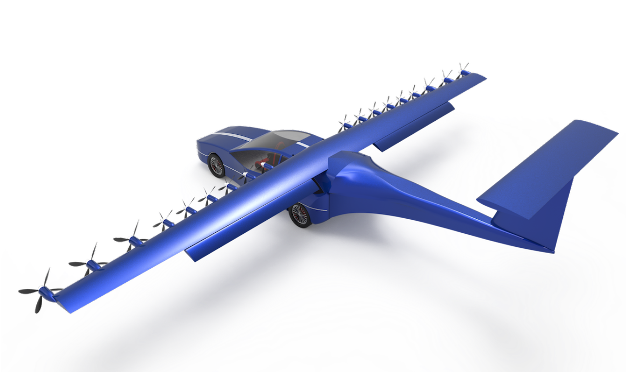
Figure 5.36: Rear view of the vehicle showing the flaps and the separate configurations
