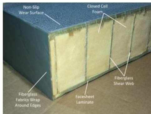
Figure 2.1: Cross-section of FRP deck
