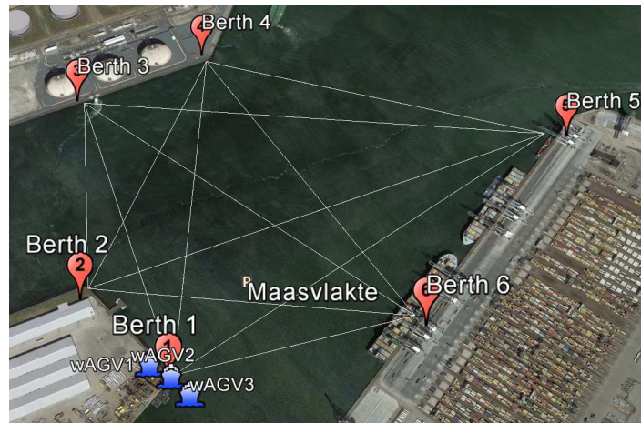
Figure 7.1: Illustration of an ITT system with six berths for three waterborne AGVs.
