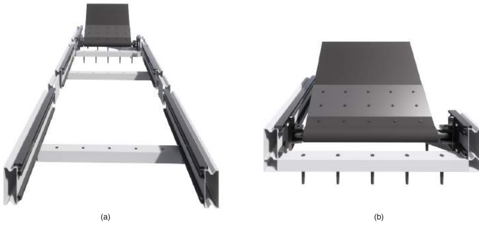
Figure [H32] Bending process, (a) plate reaches support element through sliding over rail, (b) disassembly rail.
