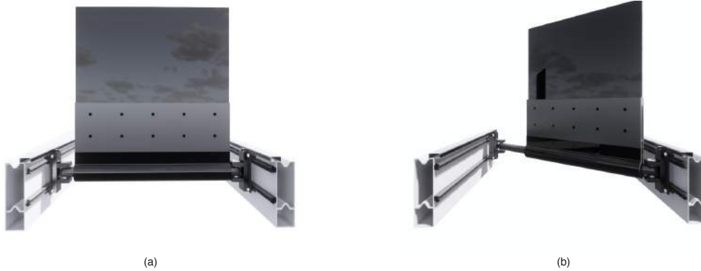
Figure [H24] Arch support free rotational motion, (a) position after bending, (b) position after torsion.
