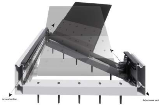
Figure [H36] Adjustment freedom within support frame four alignment of two arches.
