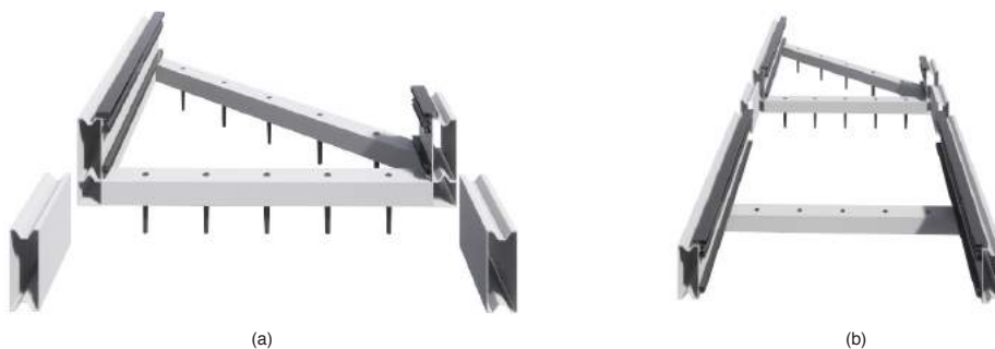
Figure [H29] Rail extension for bending deformation sequence one, (a) modular extending elements into sleeve, (b) modular one meter long rail elements.
