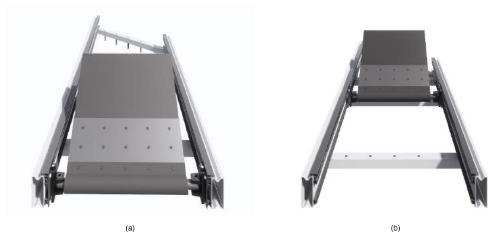
Figure [H31] Rail extension for bending deformation sequence three, (a) placement arch, (b) bending deformation over rails
