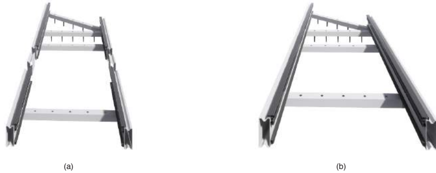
Figure [H30] Rail extension for bending deformation sequence two, (a) extension of rail for bending purposes, (b) seamless rail extension
