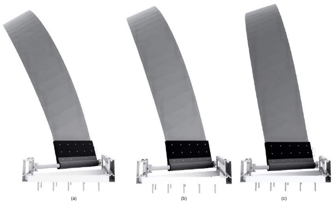
Figure [J3] Design freedom plate positions, (a) 45 degrees position, (b) 40 degrees position, (c) 35 degrees position.
