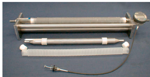
Fig. 25. Apparatus to measure the autogenous shrinkage of paste or mortar cast in a corrugated tube according to ASTM C1698, from [175].
