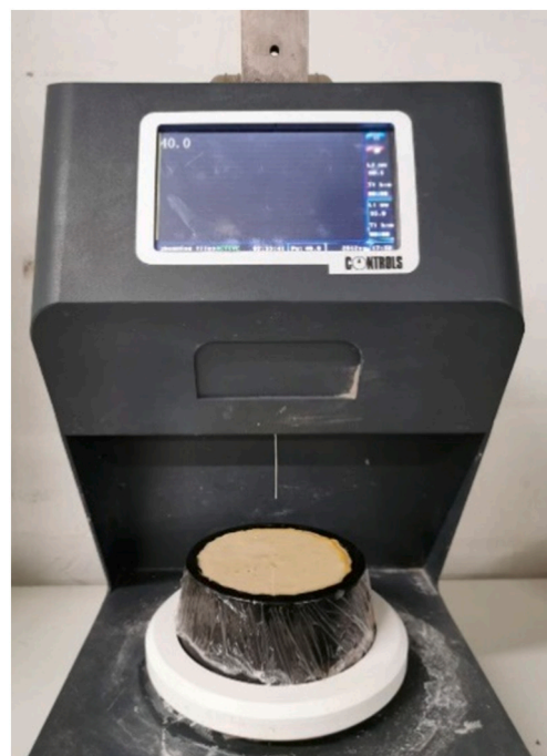
Fig. 26. Vicat apparatus to measure the setting time of AAS paste, which was sealed by plastic film, adapted from [73].
