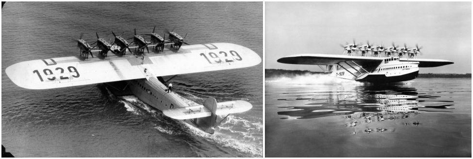
Figure 1.2: The Dornier Do-X: an early application of (distributed) over-the-wing propellers. Credits: San Diego Air and Space Museum.
