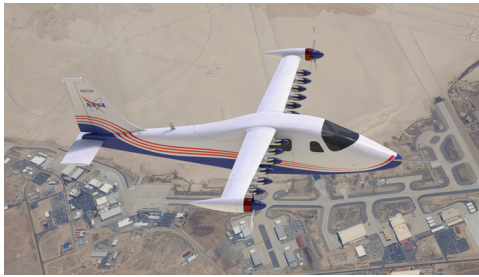
(a) NASA X-57 Maxwell [48]: tip-mounted and leading-edge distributed propulsion. Credits: NASA Langley/Advanced Concepts Lab, AMA, Inc.
