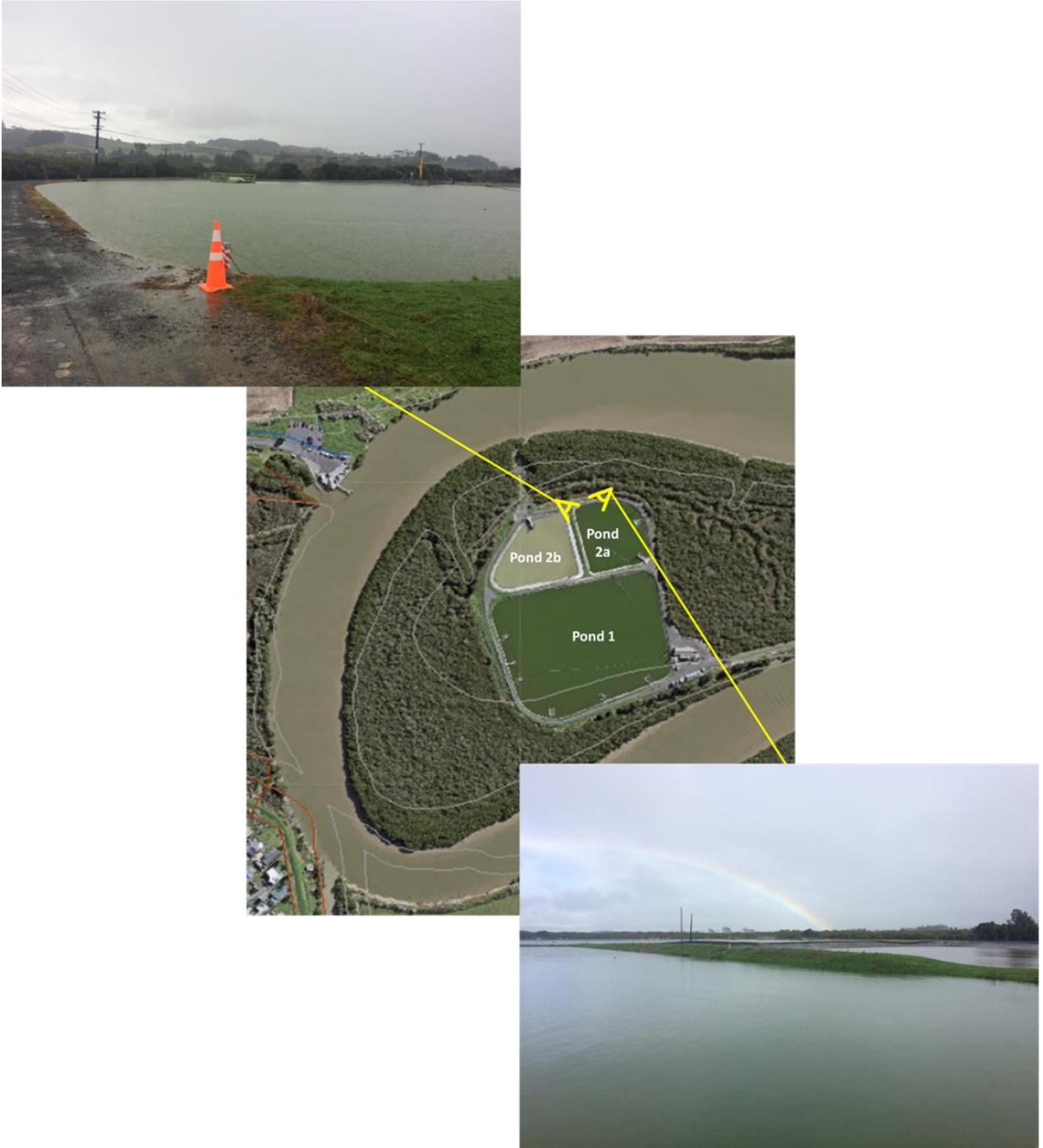
Figure 1: 7<sup>th</sup> July 2017 wet weather event (60mm over 2 days). Pond levels at 1815mm. The pond will overtop the dam embankment into the harbour at 1.85m.
