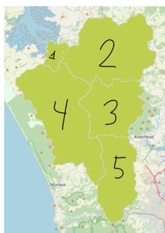
Figure 3.4: Subbasin schematization for the Kaipara river basin. Flow outside the model domain is schematized as basin 0.
