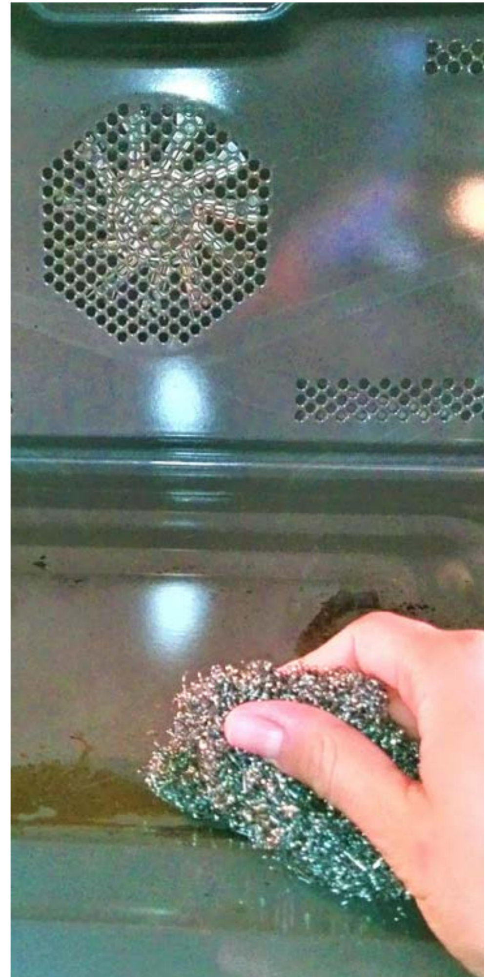
Figure 5.9 | The enamel coating can withstand more 'aggressive' cleaning materials, unlike what the user manual suggests.
