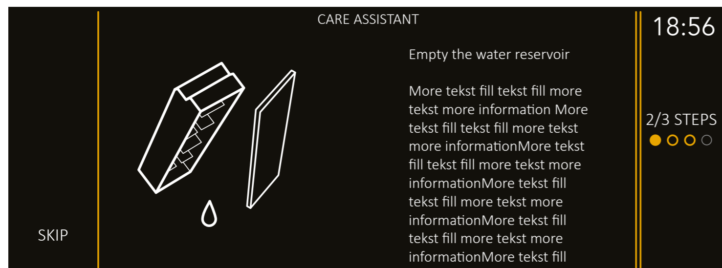
Figure 7.18 | When the door to the water reservoir is opened, the screen shows that the reservoir should be emptied.
