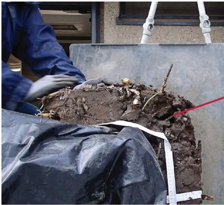
Figure 88: Normative strength in soil caused by root systems
