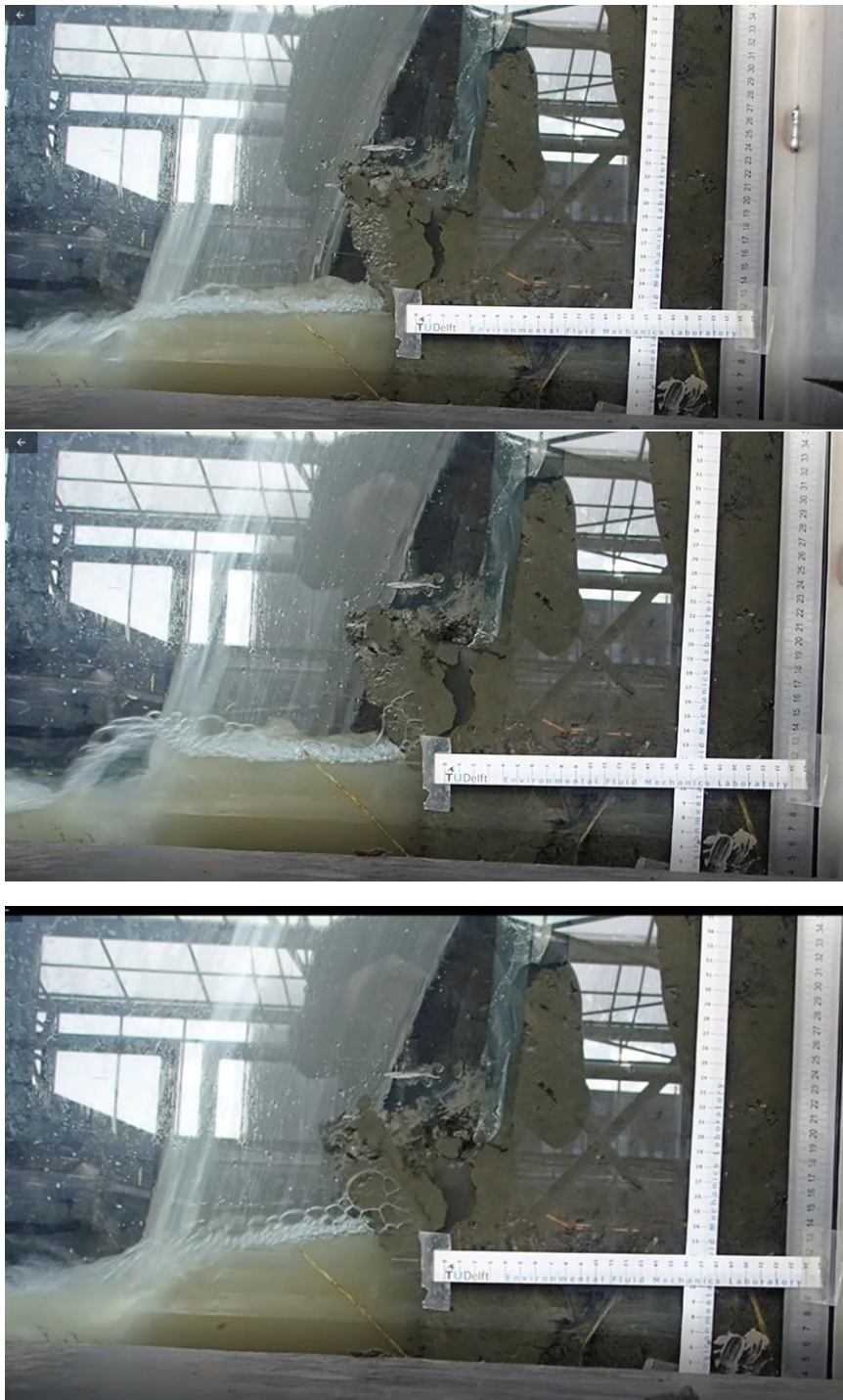
Figure 97: Rotational failure experienced at the edge of the foreland
