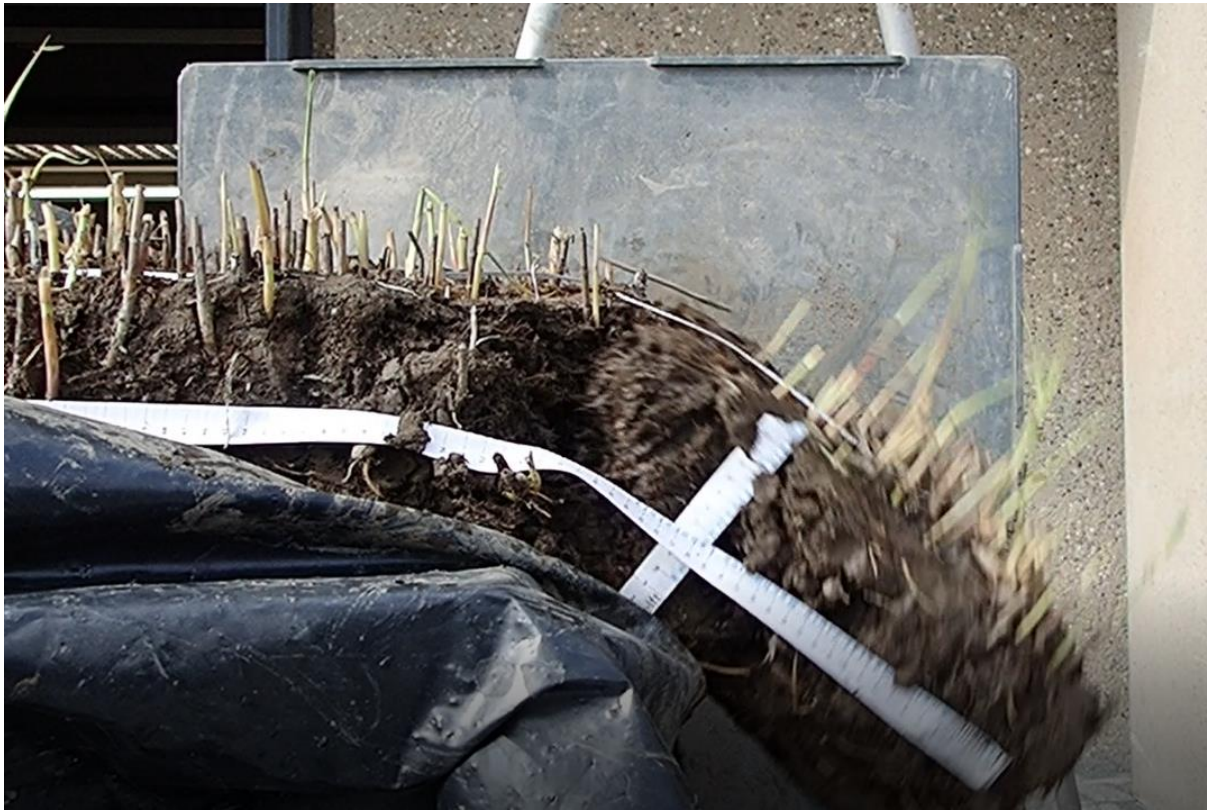
Figure 87: Clear rotational failure observed during the experiment
