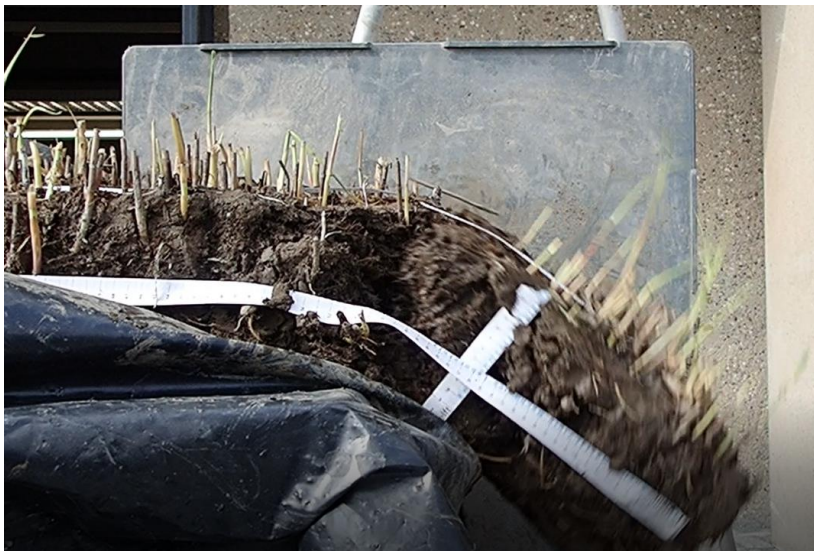
Figure 65: Rotational failure observed in the soil layer
