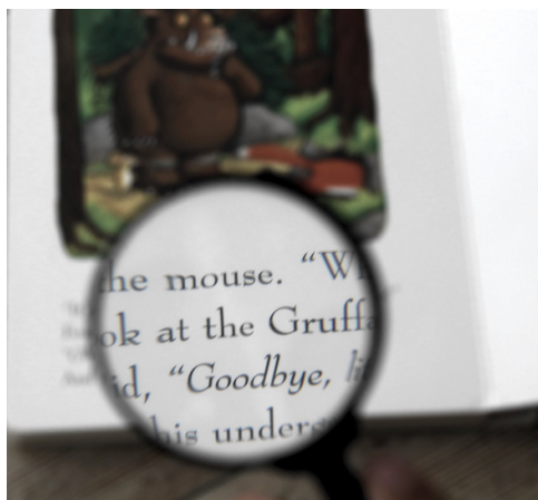
Figure 3.8: Example of a positive lens used as a magnifying glass (picture taken by A.J.L. Adam / CC-BY-SA 4.0).
