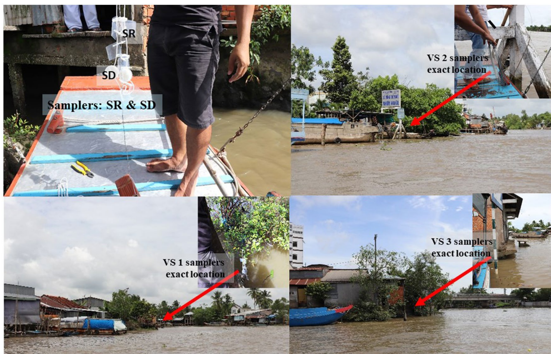
FIGURE 3 The upper left image shows the passive samplers used, which were composed of six silicon rubbers (SR) and three speedisks (SD) arranged and individually tied with tie wires and arranged in a plastic wire with brick block for added weight and support. The set was submerged in river water uninterrupted for at least 30 days in three sampling sites: images in lower left is VS1, upper right is VS2, and lower right is VS3.
