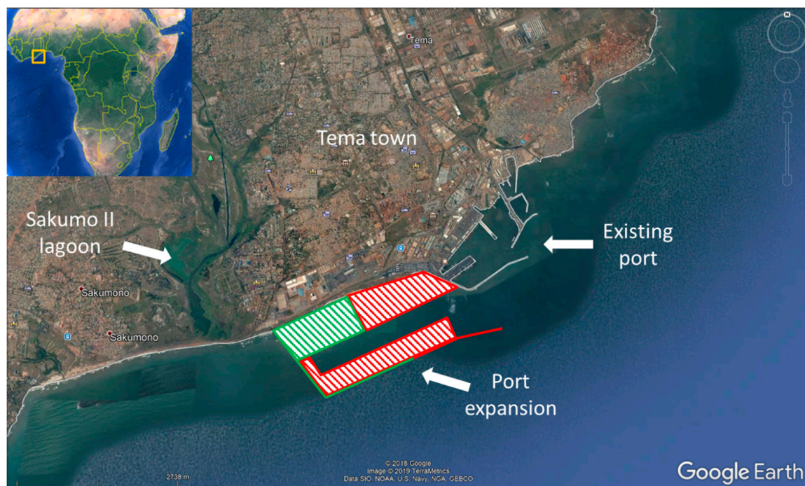
Figure 4. The location of Tema port with an indication of the realized (in green) and planned (in red) expansion to the west of the existing port and to the east of the Sakumo II lagoon (based on [63]; image source: [64]).
