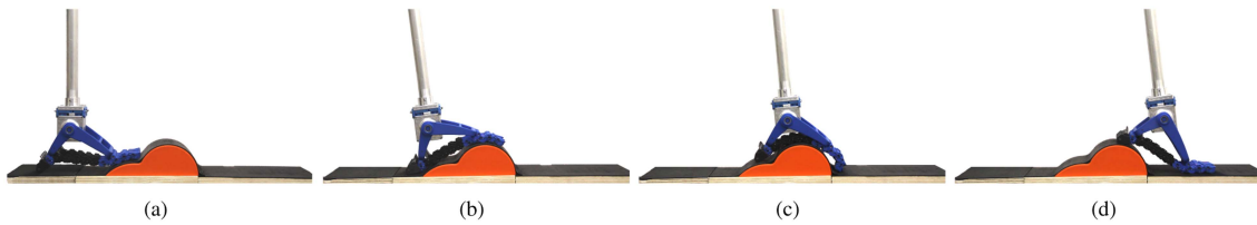
Fig. 13. Qualitative demonstration of different SoftFoot behaviors when walking on an artificial obstacle, simulating an uneven terrain: (a) initial step, where only the toes make contact with the obstacle, (b-c) stages where the entire sole is in contact, and (d) final step, where only the heel remains in contact. For this evaluation, the SoftFoot is connected to an aluminium bar and guided by an operator through the different stages of the walking.
