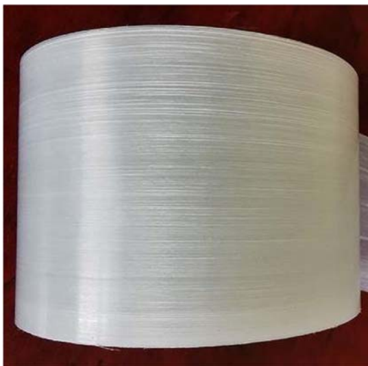
Figure 2. Prepreg tape of the FGRFP.
