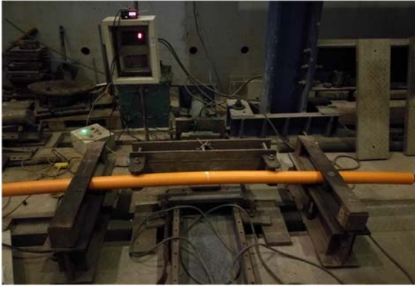
Figure 4. The four-point facility.
