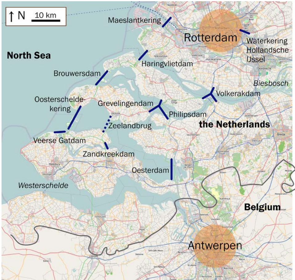
Fig. 1 The Delta works, a complex system in the Netherlands to protect the human population from flooding. The straight lines and dotted lines are gates and dams within the network. (Image courtesy of OpenStreetMap.org .)
