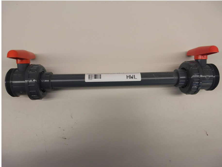
Figure 4: Segment of a pipe used in the experiment. With valves that can close and open at each end.
