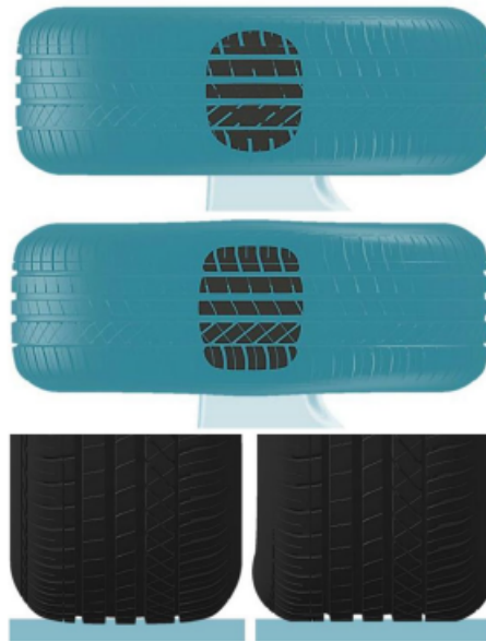
Figure 2.15: Comparison of undeformed and deformed tire with fully treaded surface by Mortazawy et al. [44].
