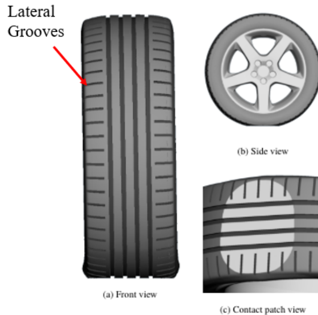
Figure 3.1: Deformed tire with lateral and longitudinal grooves tested by Hobeika and Sebben [28].
