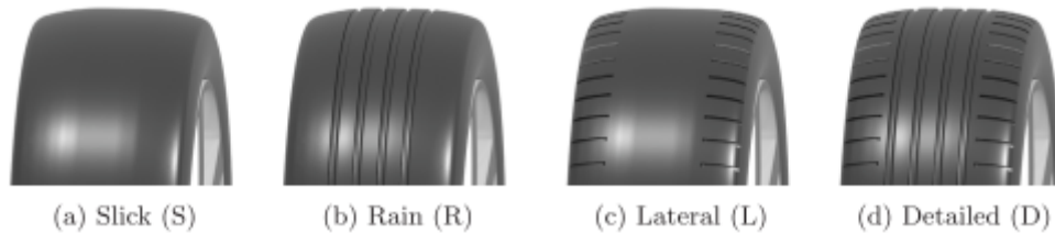
Figure 2.11: Tire surface geometries tested by Josefsson et al. [30, 32] : (a) smooth tire surface; (b) longitudinal grooves tire surface; (c) lateral grooves tire surface; (d) lateral and longitudinal grooves, approximating a treaded tire surface.
