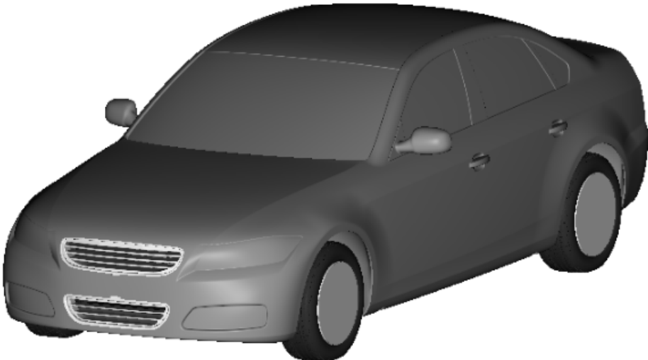
Figure 8.4: ISO-View of DrivAer model used for the full vehicle tests.
