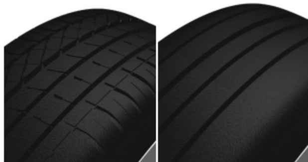
Figure 2.12: Fully treaded tire surface (left) and grooved tire surface (right) by Alajbegovic et al. [36].
