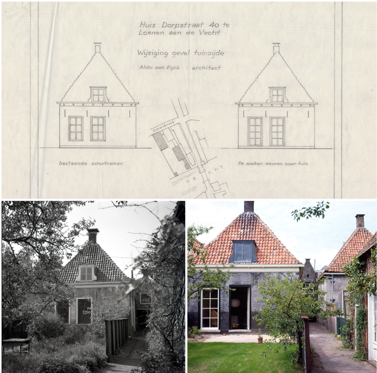
Figure 16. (Left) Elevation and site plan, courtesy of The Aldo and Hannie van Eyck Foundation; (Right) garden façade before and after transformation, photographed by Aldo van Eyck, courtesy of The Aldo and Hannie van Eyck Foundation
