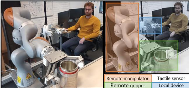
Fig. 5: Overview of the teleoperated gripper setup. The user controls the remote robot with the local haptic device, the SIGMA7. The remote robot exists out of a manipulator, the KUKA iiwa7, with at the end effector a gripper, the FUSE gripper. For tactile feedback, the remote gripper has tactile sensors, the ChromaTouch, on the gripper fingers.
