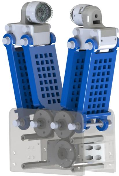
Fig. 2: 3D render of the 2nd iteration FUSE gripper
